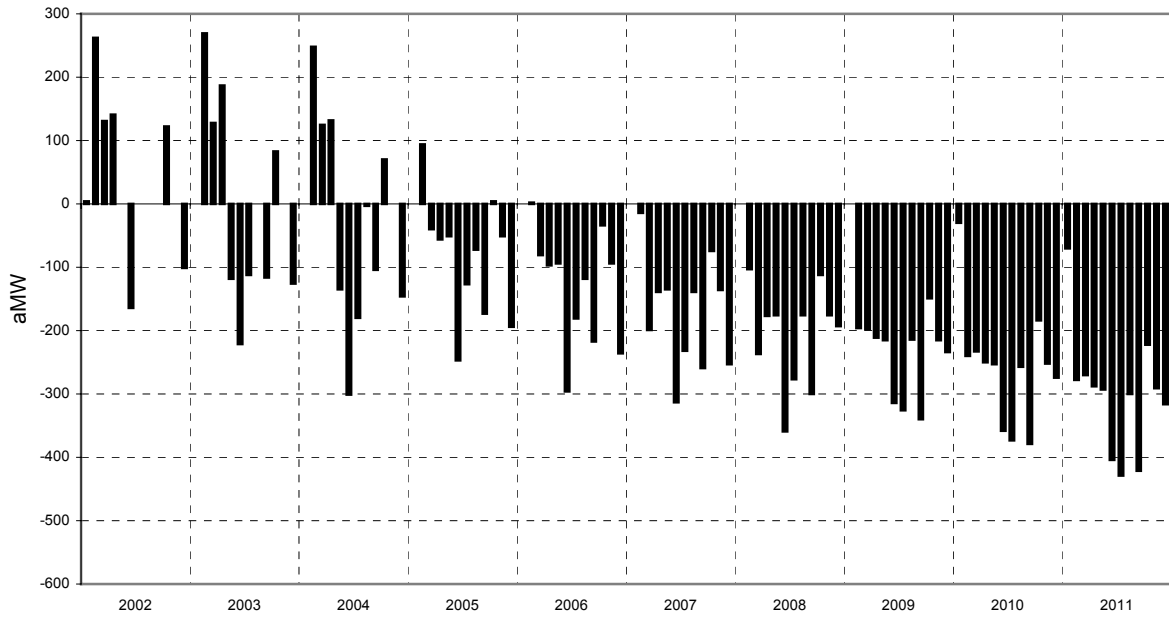
Figure 6 Monthly Energy Surplus / Deficiency 90 th Percentile Water, 70 th Percentile Load, Existing Resources with Garnet
