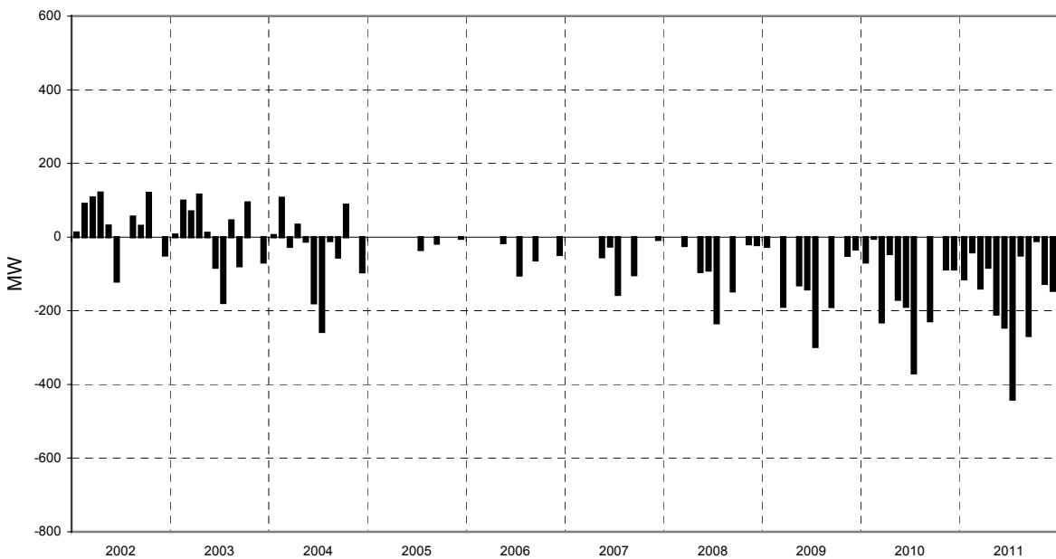
Figure 16 Monthly Peak-hour Surplus / Deficiency 90 th Percentile Water, 70 th Percentile Load, Strategy 4 Resources with Garnet
