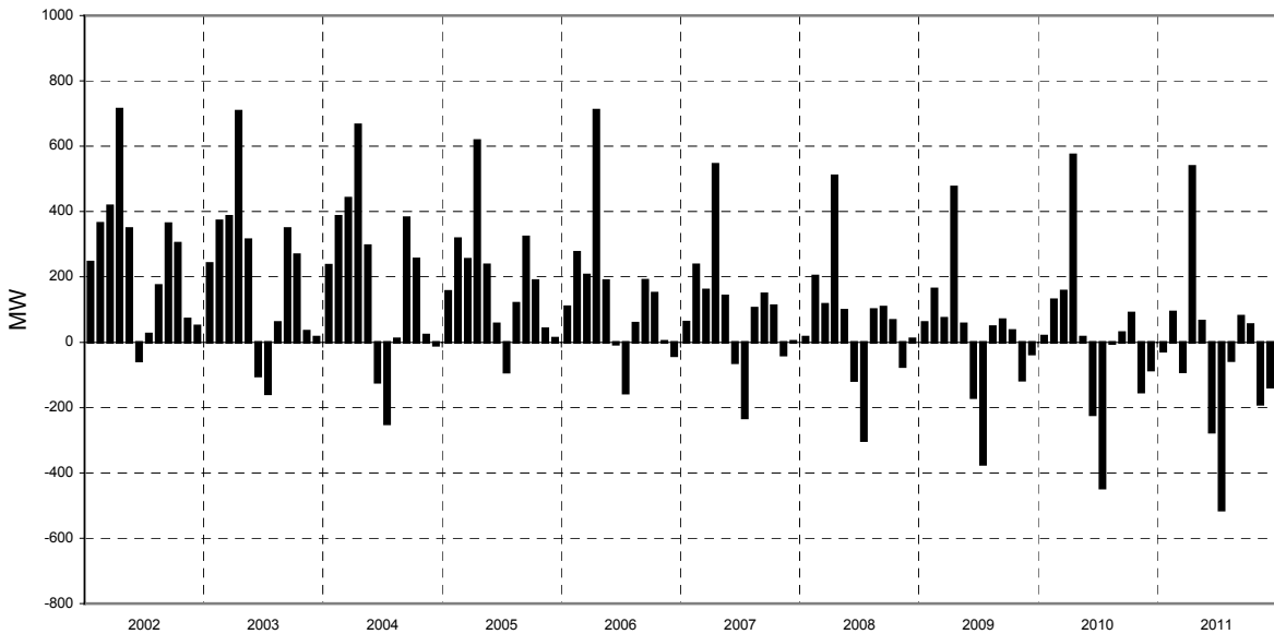
Figure 3 Monthly Peak-hour Surplus / Deficiency Median Water, Median Load, Existing Resources with Garnet
