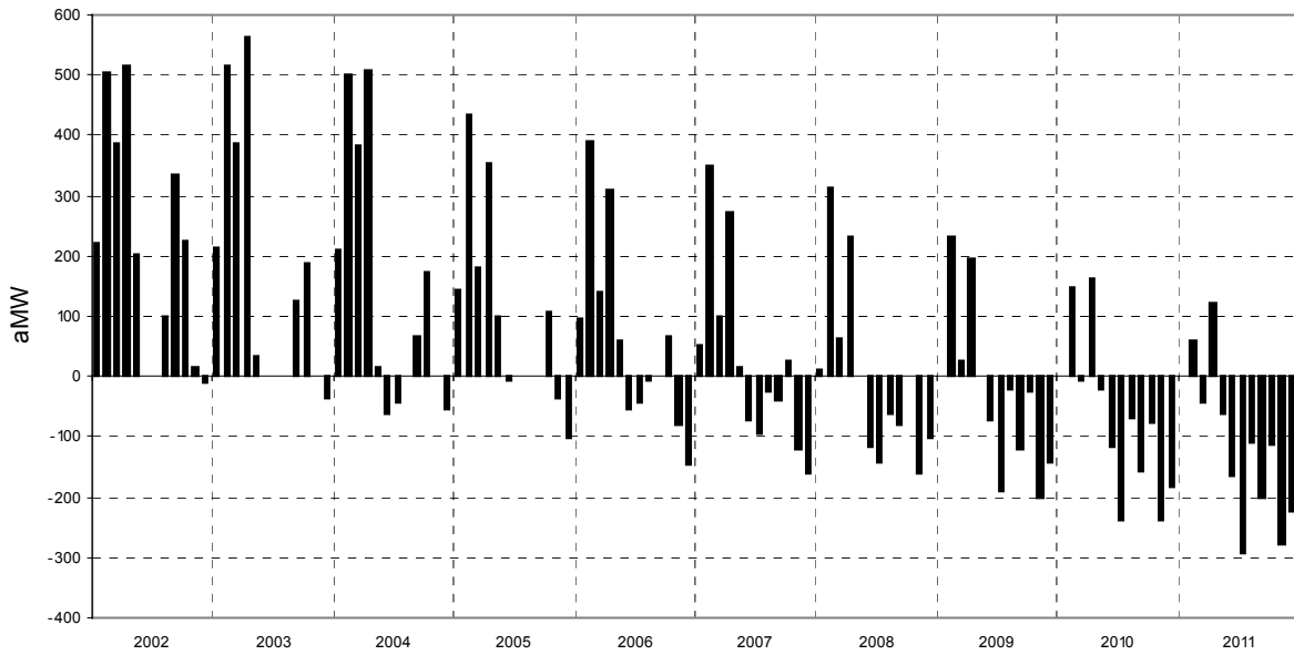
Figure 4 Monthly Energy Surplus / Deficiency 70 th Percentile Water and Load, Existing Resources with Garnet
