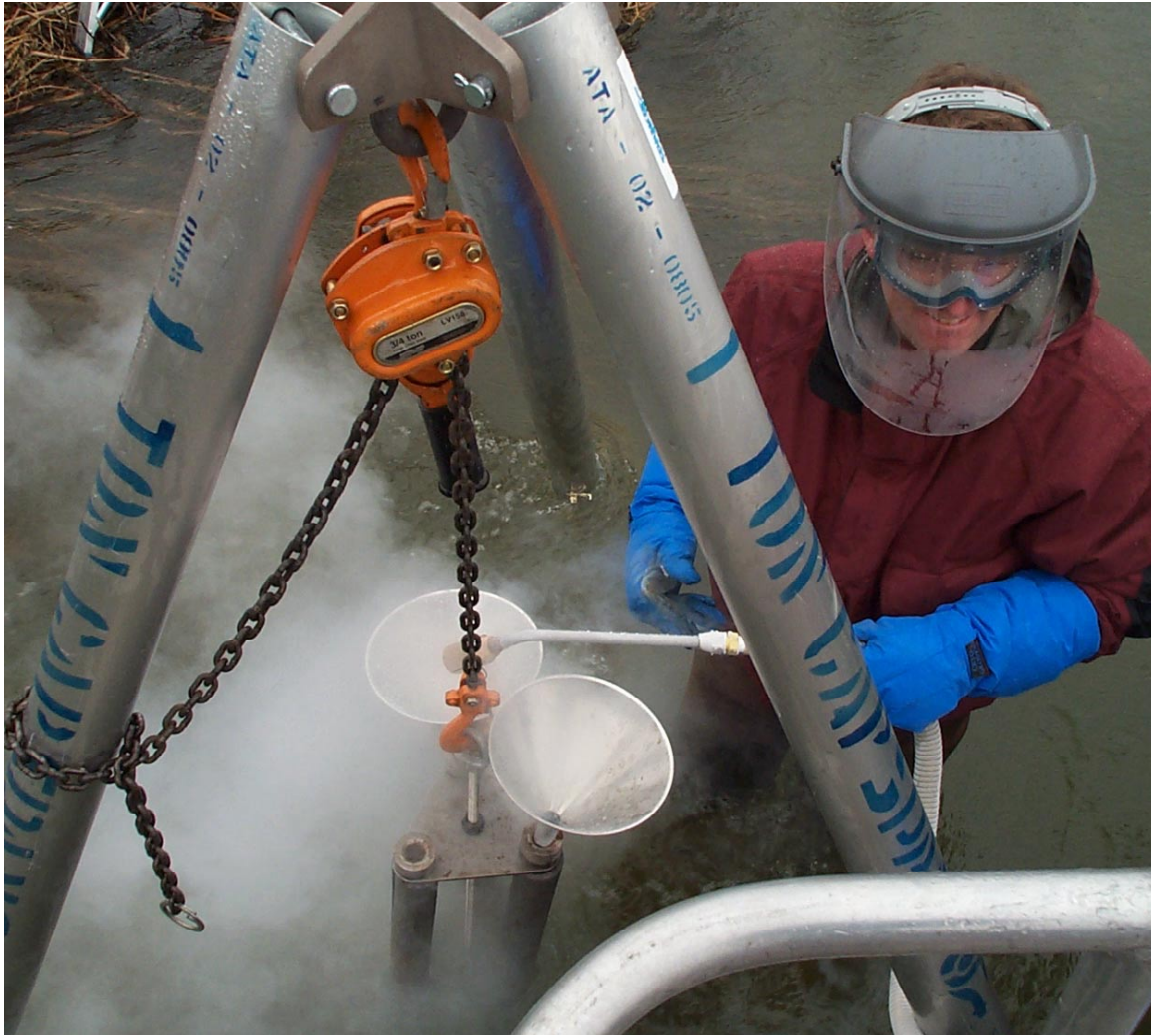
Figure 40. Tri-tube assembly, tripod, and chain hoist used for extracting freeze cores. Liquid nitrogen is poured down into the tubes through the funnels to freeze the bed.
