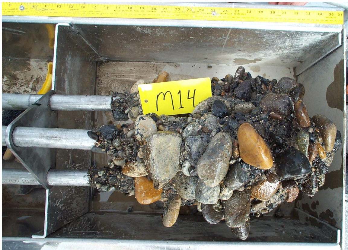
Figure 42. The surface layer of the sediment core is lost due to thawing. The triangular plate at left was at the riverbed surface.
