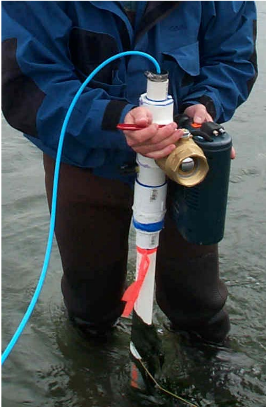
Figure 46. The piezometer is outfitted with a pressure-regulating ball valve device and a small electric air compressor.
