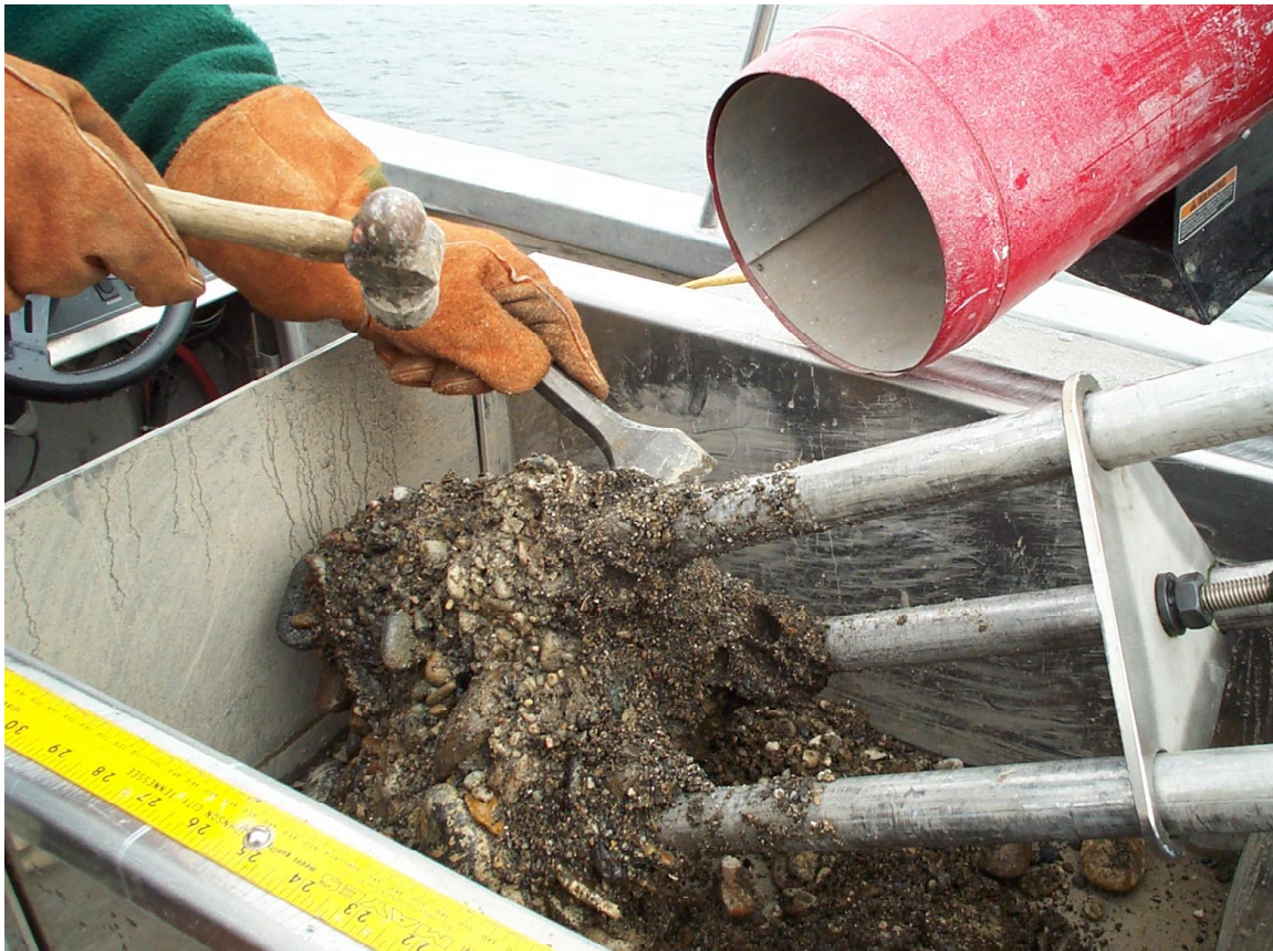
Figure 41. Thawing the freeze core over an aluminum sample collection box with a portable propane heater.
