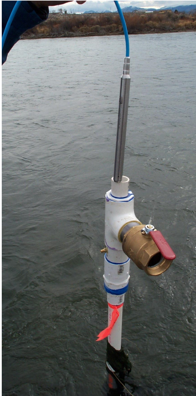
Figure 45. The data logger is inserted into the piezometer through the pressure-regulating device.
