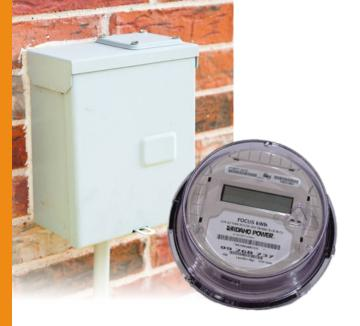
The transfer switch is very important. If your generator is running and its output is not completely separated from Idaho Power's system, your generator will feed power back into Idaho Power's line through the transformer that provides you with power. The transformer will step up the current to the normal line voltage, which could be as high as 34,500 volts. An unsuspecting line worker, working on what they think is a deactivated line, could be killed.
