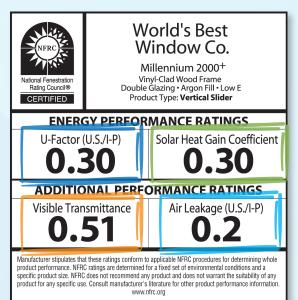
Low emissivity (low-E) coatings can help decrease the U-Factor, the SHGC and UV sun damage to floors, carpets and furniture. A low-E coating is a microscopically thin layer of metal or metal oxide deposited on window glass. It reflects warmth back into the home in the winter and prevents unwanted rays from entering the home in the summer.
