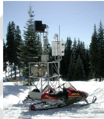
Cloud seeding ground generator.
