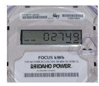
The letters "kWh" indicate the Focus meter is displaying energy usage data. In this example, the customer's energy usage is 2749 kWh.
