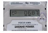
The letters "PD" are visible when the Focus meter displays peak demand data. In this example, peak demand is 6.87 kW.
