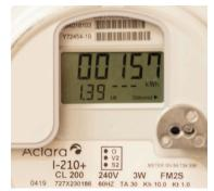
The Aclara meter shows peak demand data on the same display setting as energy usage. Peak demand is the bottom number. In this example, peak demand is 1.39 kW. **ENERGY FLOW:** Dashes or arrows in the display show when energy is being delivered to you and, if you generate energy at your home or business through rooftop solar panels, for example.
