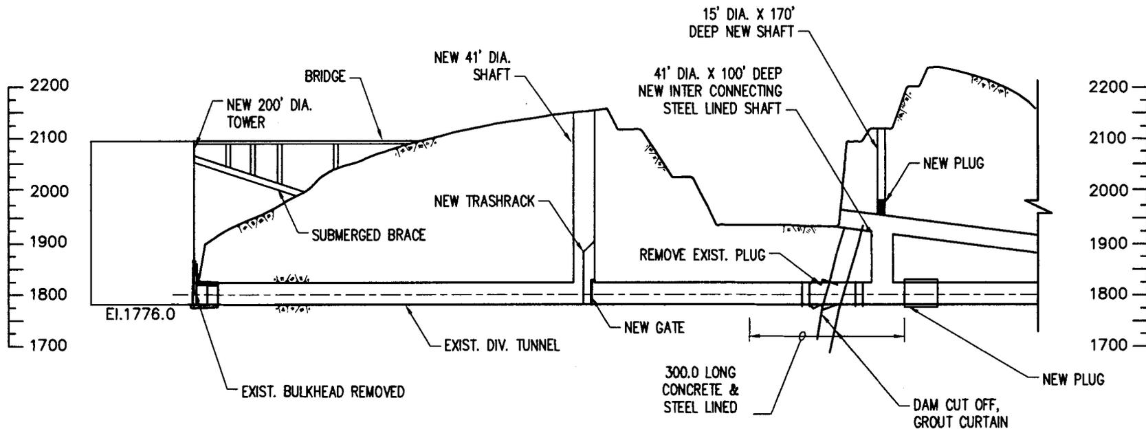
DEVELOPED PROFILE ON  $\phi$  EXIST. TUNNEL
