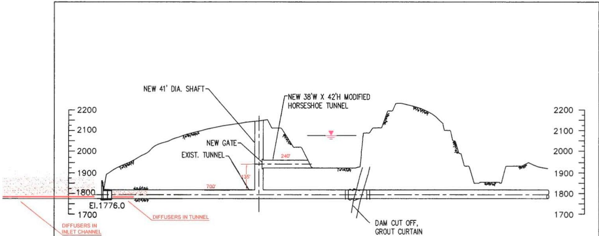
DEVELOPED PROFILE ON  $\bar{C}$  EXIST. TUNNEL
