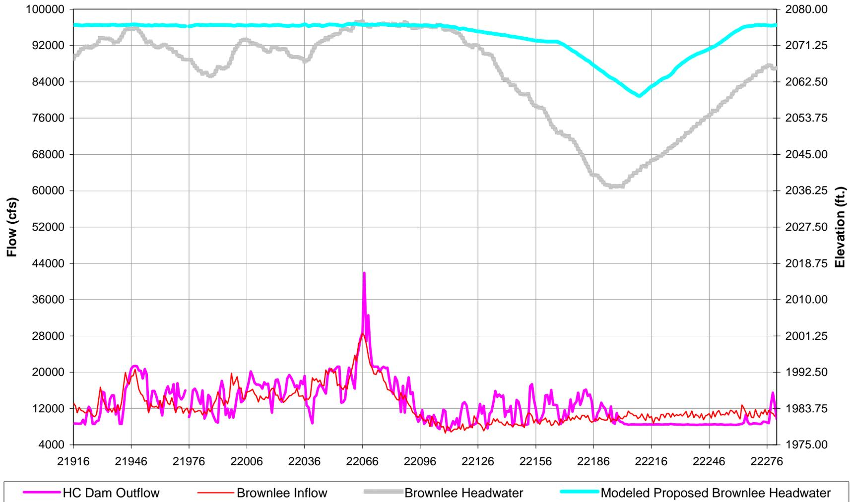
Figure 6. Operational details for Brownlee Reservoir, 2003.
