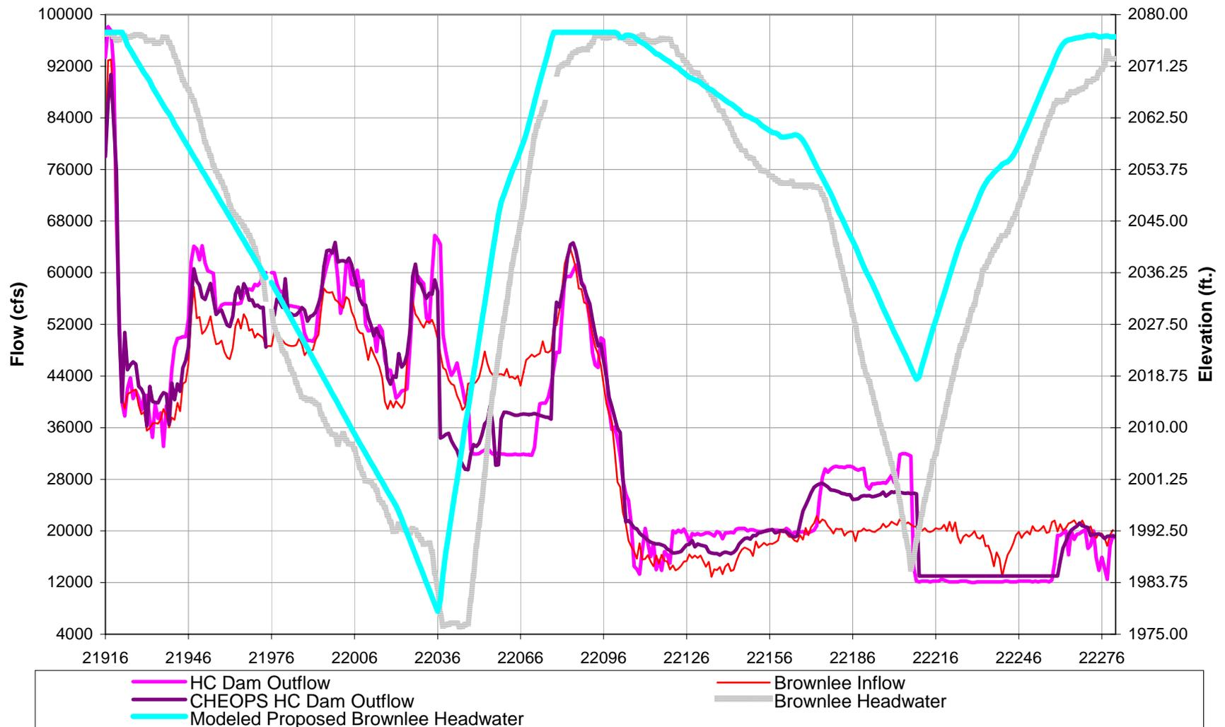
Figure 3. Operational details for Brownlee Reservoir, 1997.
