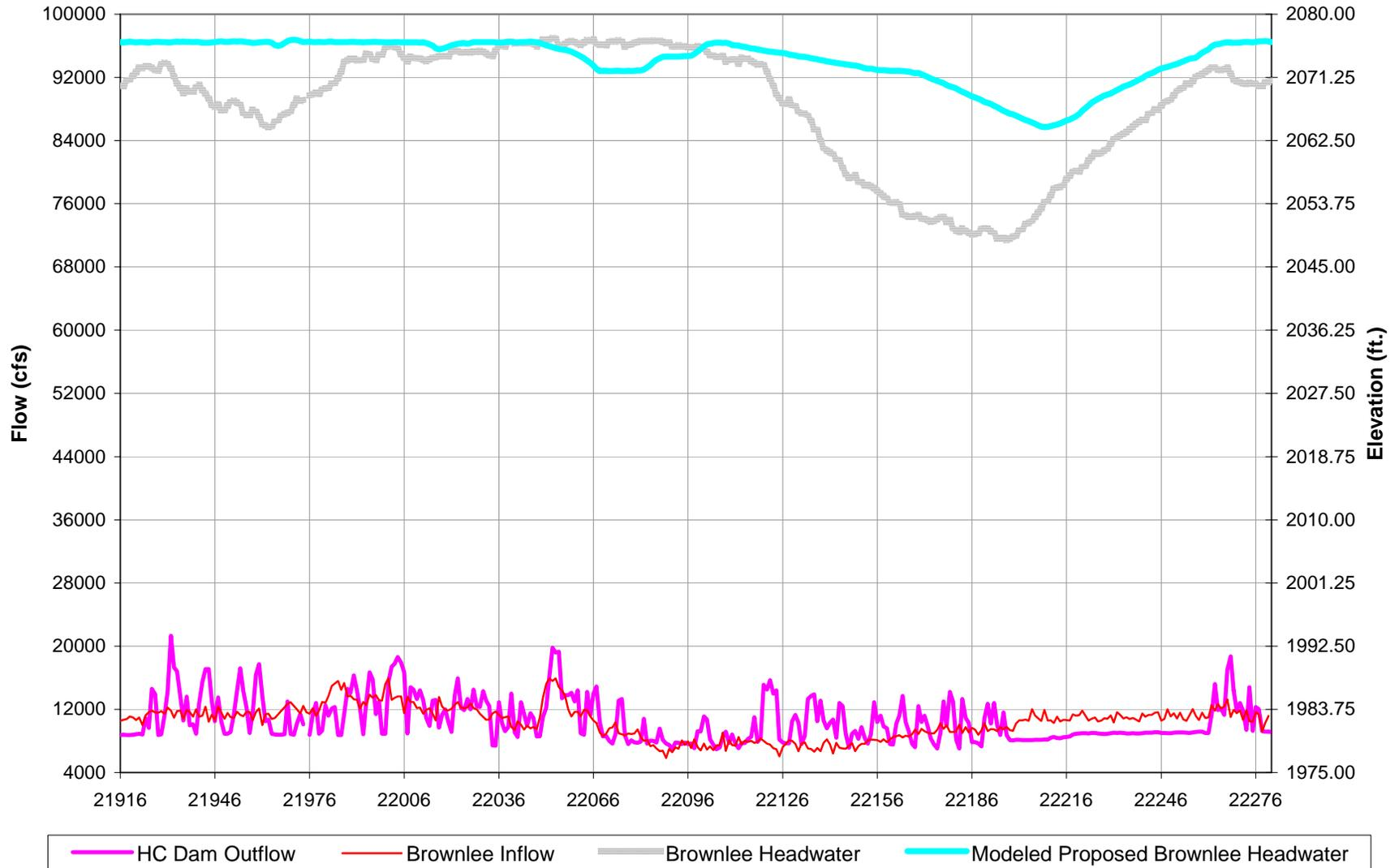
Figure 4. Operational details for Brownlee Reservoir, 2001.
