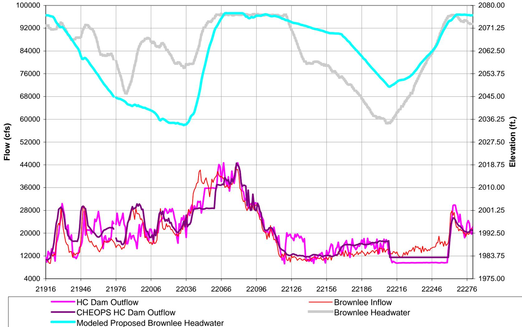
Figure 1. Operational details for Brownlee Reservoir, 1995.
