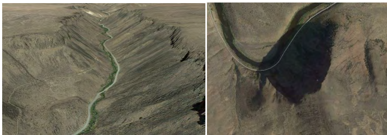
Figure 14: Situations where steep slopes and topographic shade, respectively, would lead to exclusion from thermal modeling.
