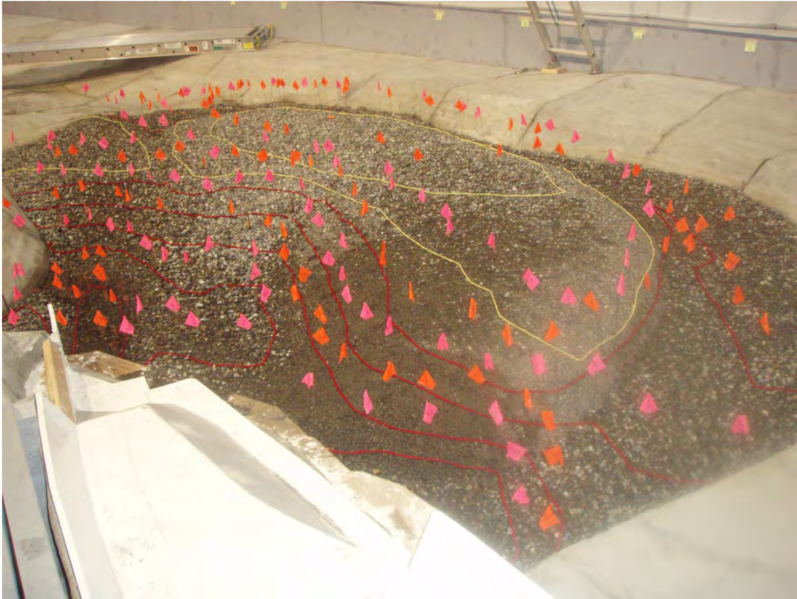
Photo 1 – post 70 Kcfs scour test with deflector concept 20 and training wall in place
