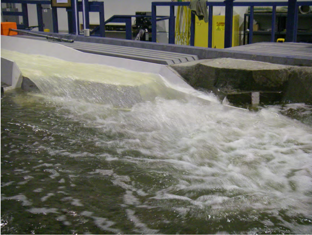
Photo 6.3.3 Final Documentation, Deflector 20, 60,000 cfs, 1704.2' tailwater.
