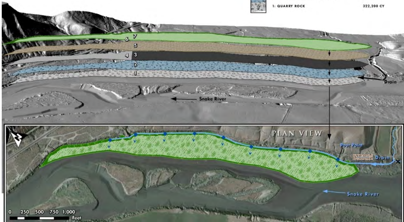
Figure 8: Potential emergent wetland with surface flow at a drain site near Walters Ferry (RM 440).
