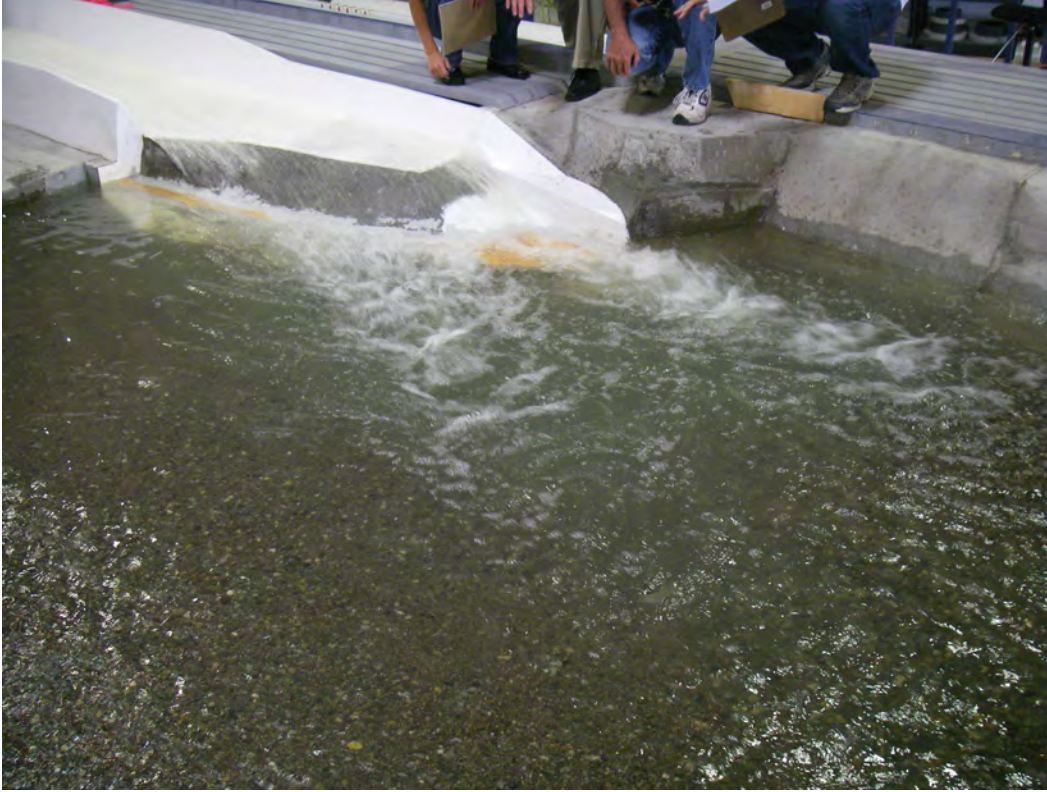
Photo 6.2.3 Generic Deflector Concept 3 - June 12, 2007 Witness Test
