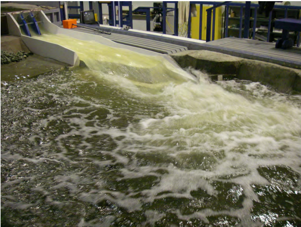
Photo 6.3.4 Final Documentation, Deflector 20, 100,000 cfs, 1708.4' tailwater.
