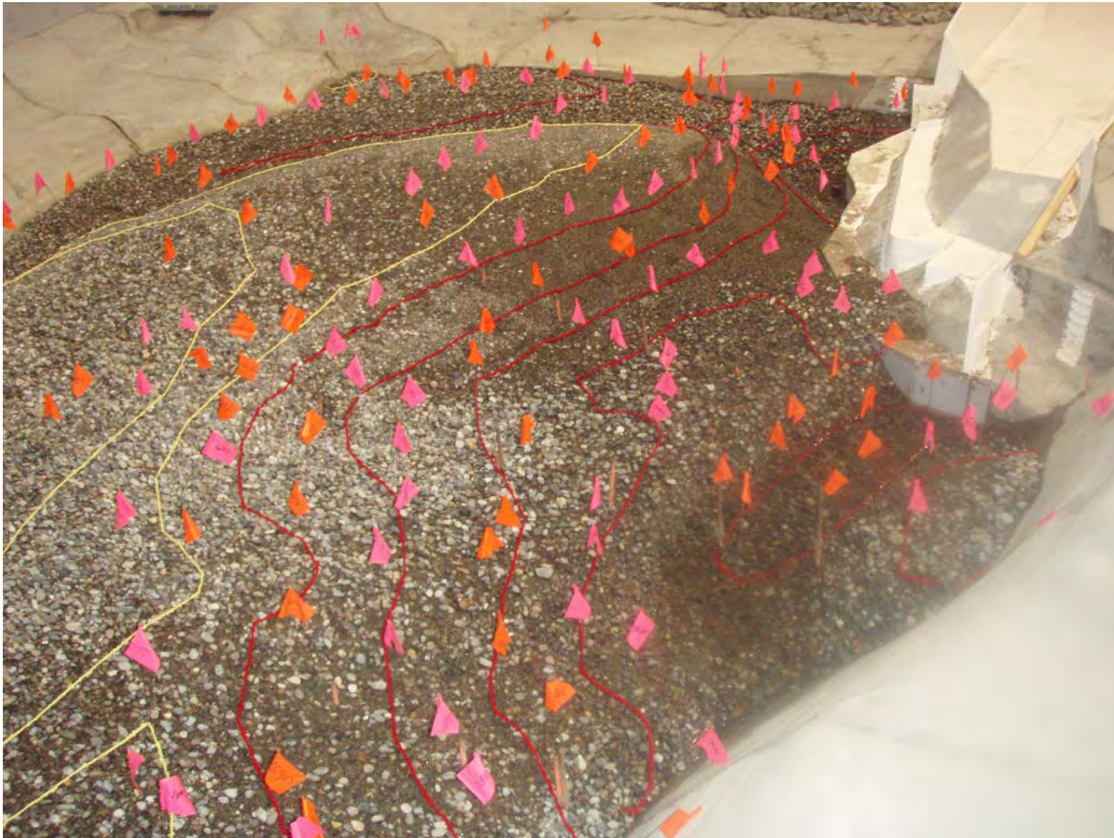
Photo 2 – post 70 Kcfs scour test with deflector concept 20 and training wall in place
