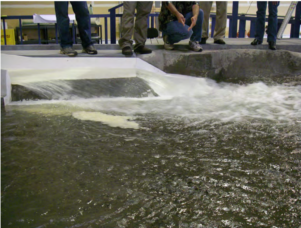
Photo 6.2.2 Generic Deflector Concept 2 - June 12, 2007 Witness Test
