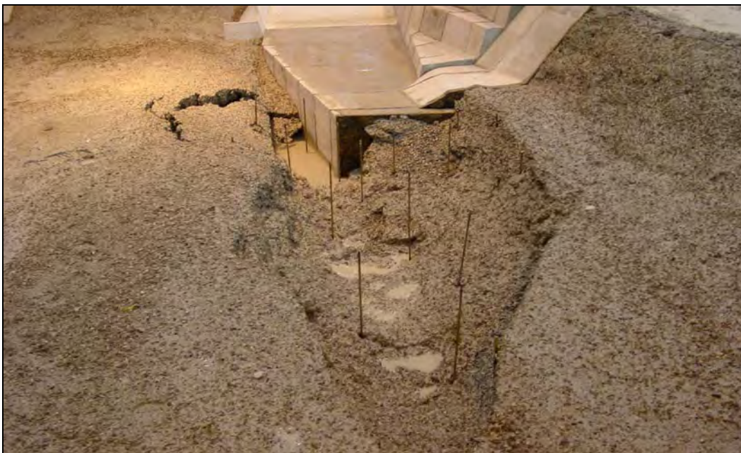
Figure 4-6. Primary scour hole looking upstream to apron after the scour test without deflector (IP-3D-06)
