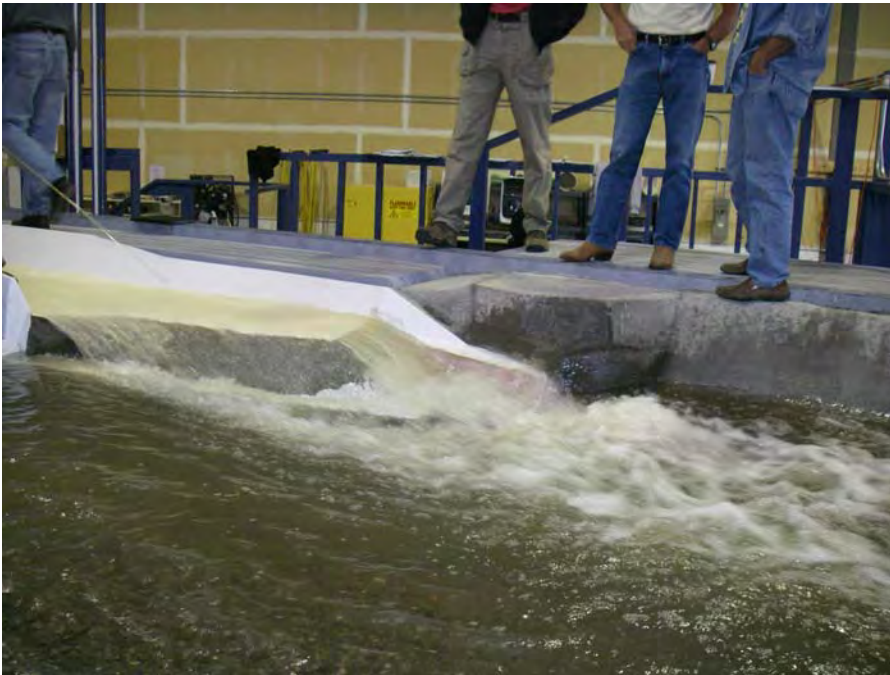
Photo 8 – Deflector Test 40 kcfs
