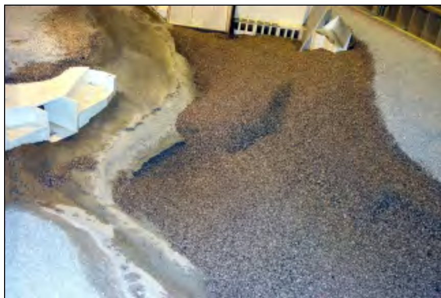
Figure 4.36. Looking upstream after 40 kcfs per crest gate
