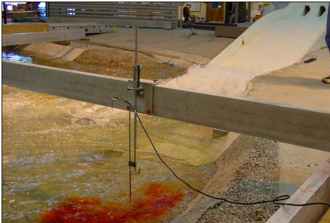
Figure 5-16. Photograph of wave height instrumentation during model test
