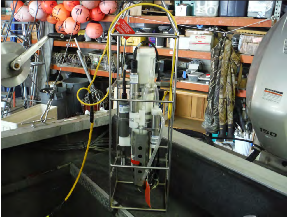
Figure 3. Sea-Bird Electronics, Inc. SEACAT Profiler CTD SBE-19plus, used to collect water column profiles of temperature, dissolved oxygen, and specific conductance in Brownlee Reservoir near Oxbow, Oregon, May 7–9, 2012.
