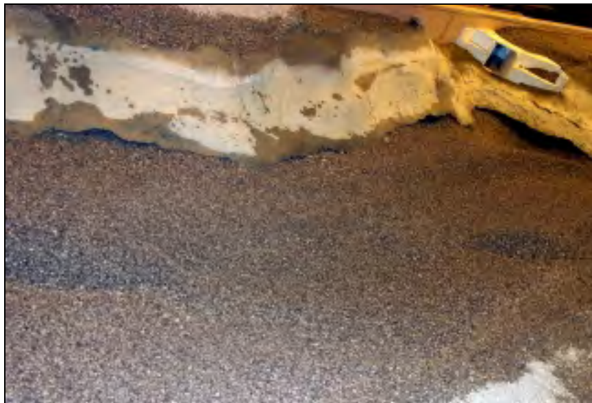
Figure 4.71. Scour patterns downstream
