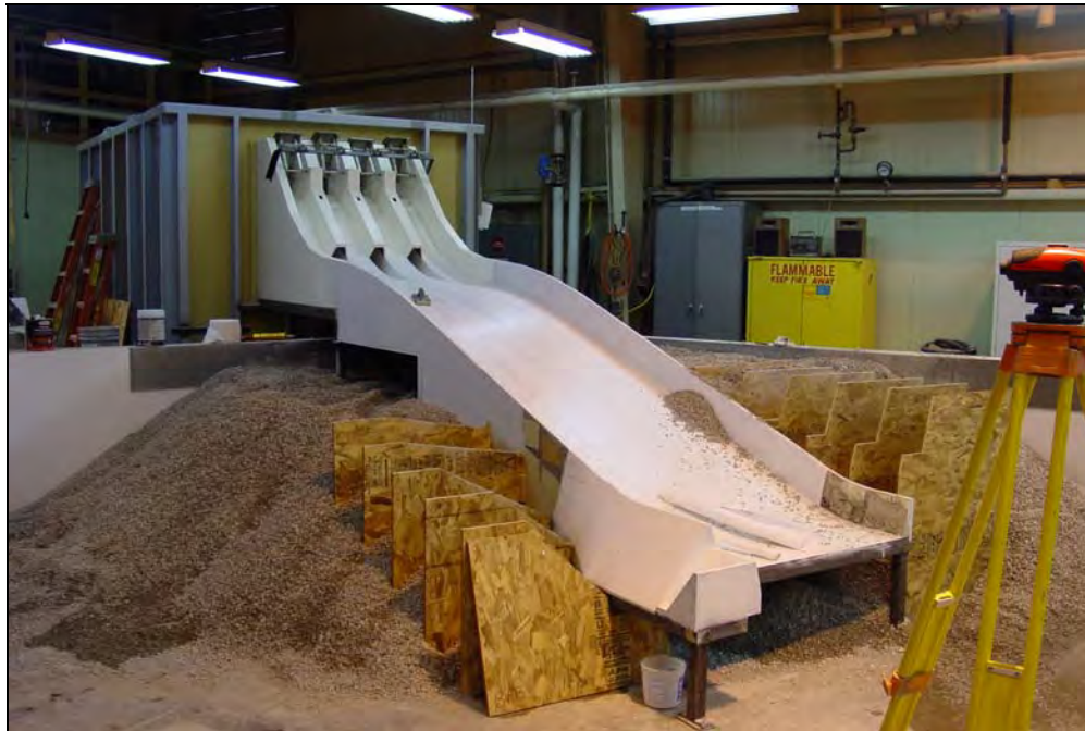
Figure 2-3. Photograph of spillway during model construction
