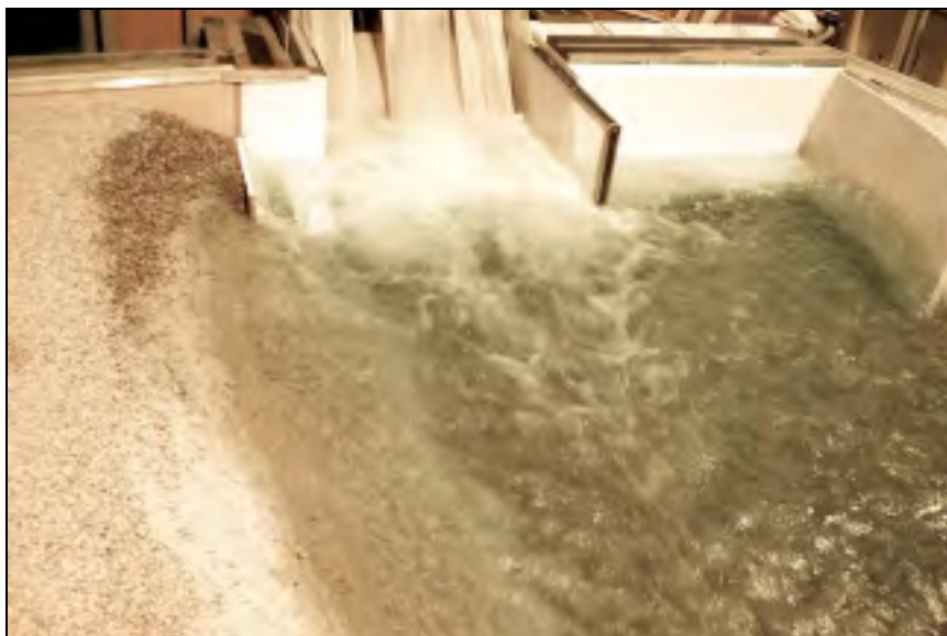
Figure 4.20. Spillway jets at 10.0 kcfs per crest gate
