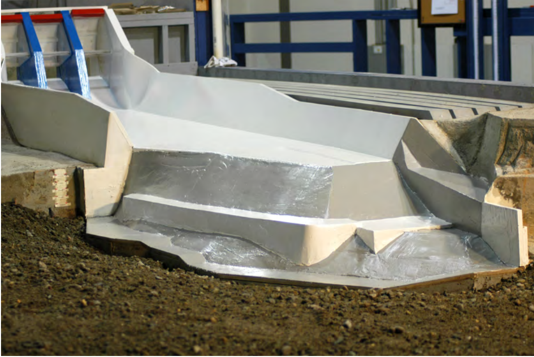
Photo 6.2.17 Deflector 20, Dry, Recommended Design
