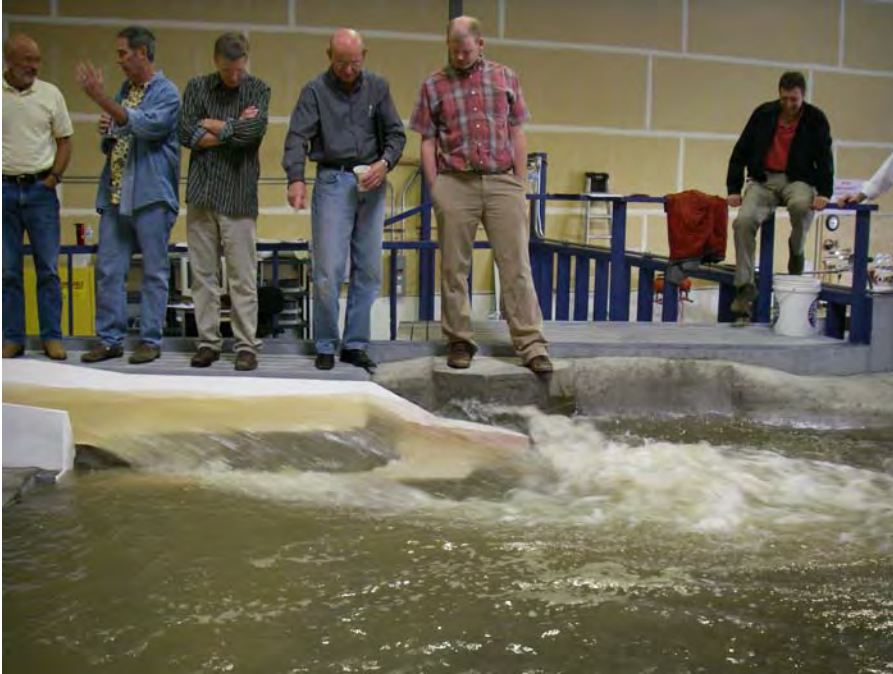
Photo 10 – Deflector Test 100 kcfs
