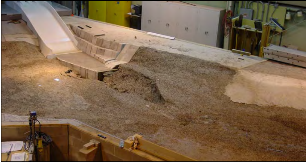
Figure 4-5. Photograph of the bed after the scour test without deflector (IP-3D-06)
