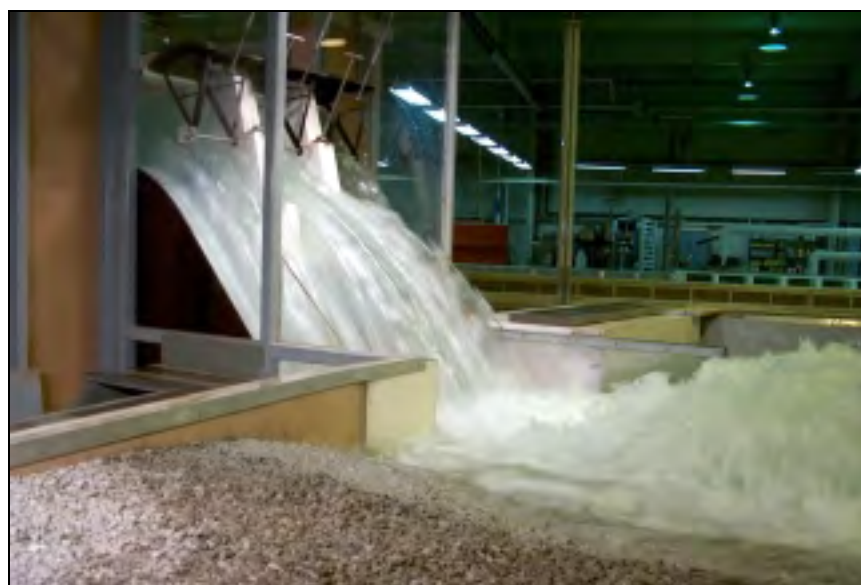
Figure 4.51. Stilling basin during design discharge
