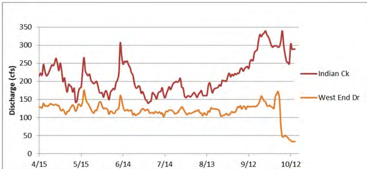
Figure 4a. 2017 daily average inflow data for Indian Creek at Kimball (RC1.8) and West End Drain (RC8.1).
