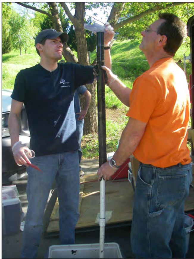
Figure 8. Extraction process used to subsample bed-sediment cores collected from Brownlee Reservoir near Oxbow, Oregon, May 7–9, 2012.
