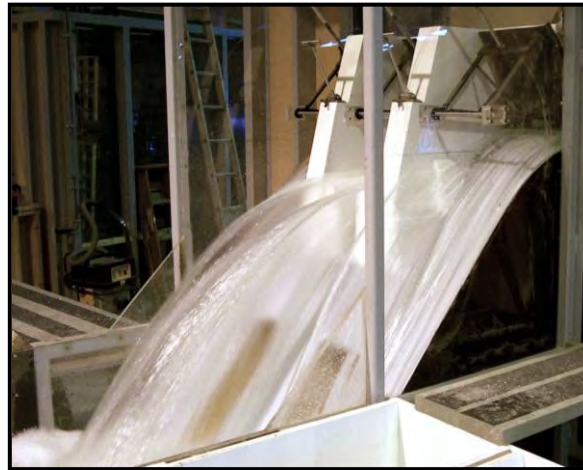
Figure 4.1 Unattached Spillway Jet
