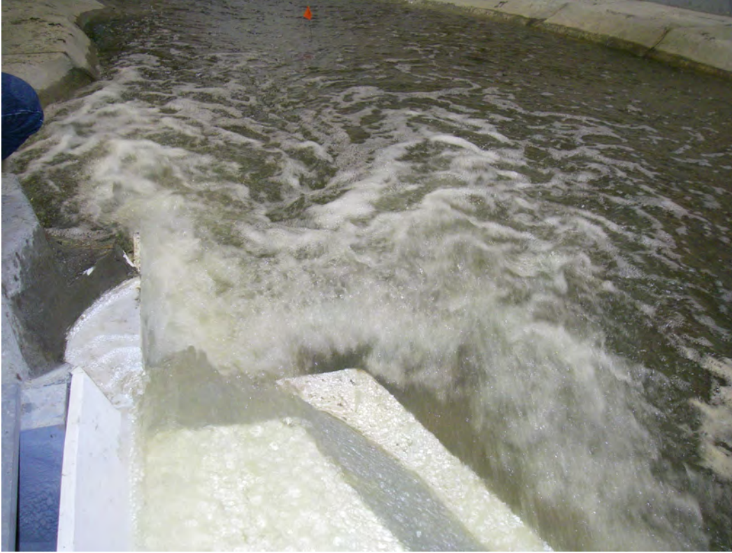
Photo 6.2.19 Deflector 21, 40,000 cfs, Low Tailwater, 3-Bay Operation
