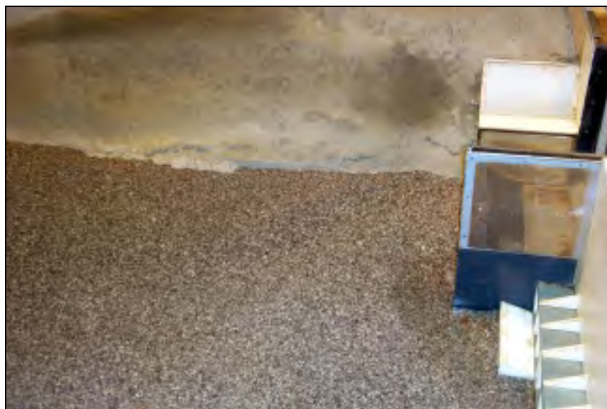
Figure 4.27. Tailrace scour after 20 kcfs per crest gate
