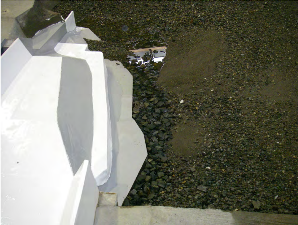
Photo 6.2.22 Rip rap test, Deflector 20, 20,000 cfs, 4'-6' rip rap
