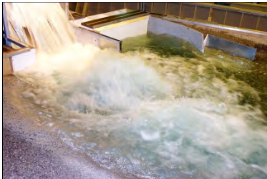
Figure 4.46. Spillway jets at 67 kcfs per crest gate
