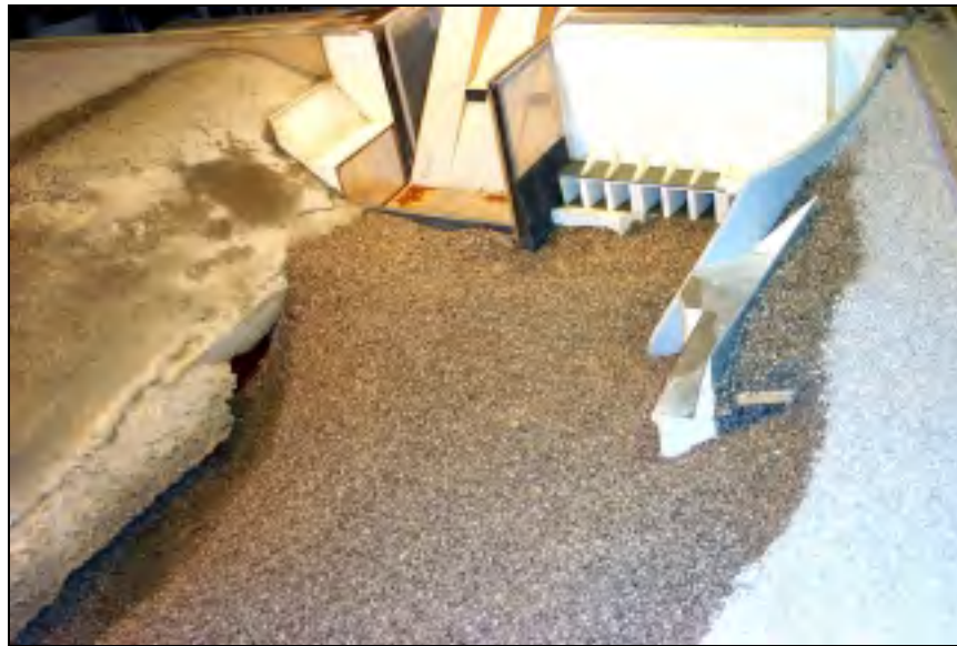
Figure 4.41. Right bank scour after 50 kcfs per crest gate
