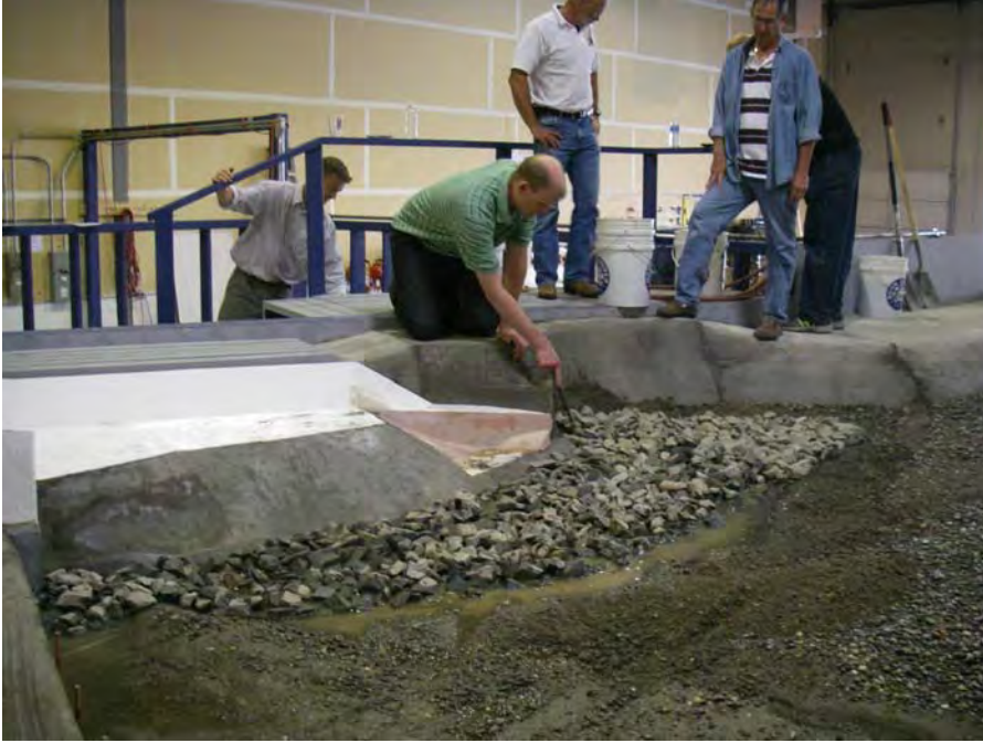
Photo 4 – Plunge Pool Riprap Test
