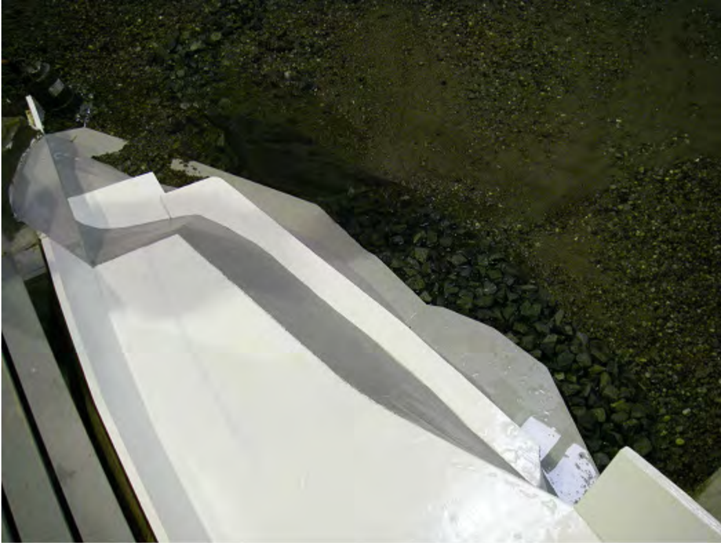
Photo 6.2.23 Rip rap test, Deflector 20, 40,000 cfs, 4'-6' rip rap.
