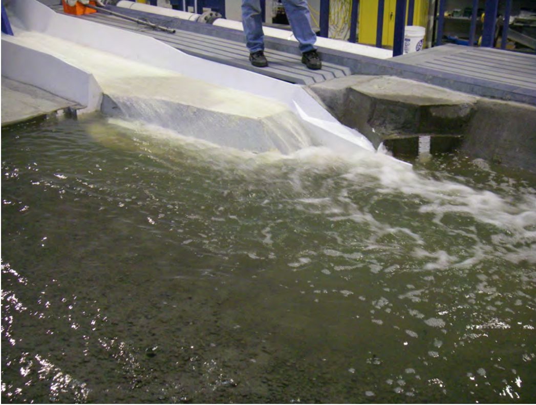
Photo 6.3.1 Final Documentation, Deflector 20, 20,000 cfs, 1697.2' tailwater.
