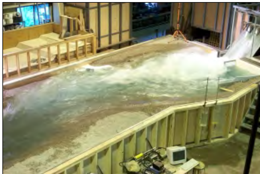
Figure 4.66. Overall flow pattern of design discharge with deflectors
