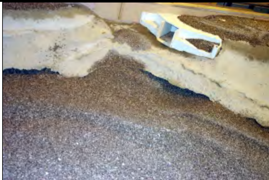
Figure 4.60. Scour hole near diversion tunnel
