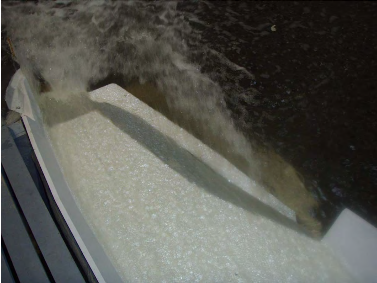
Photo 2 – Arrangement 20 – 40 Kcfs – 3 gates
