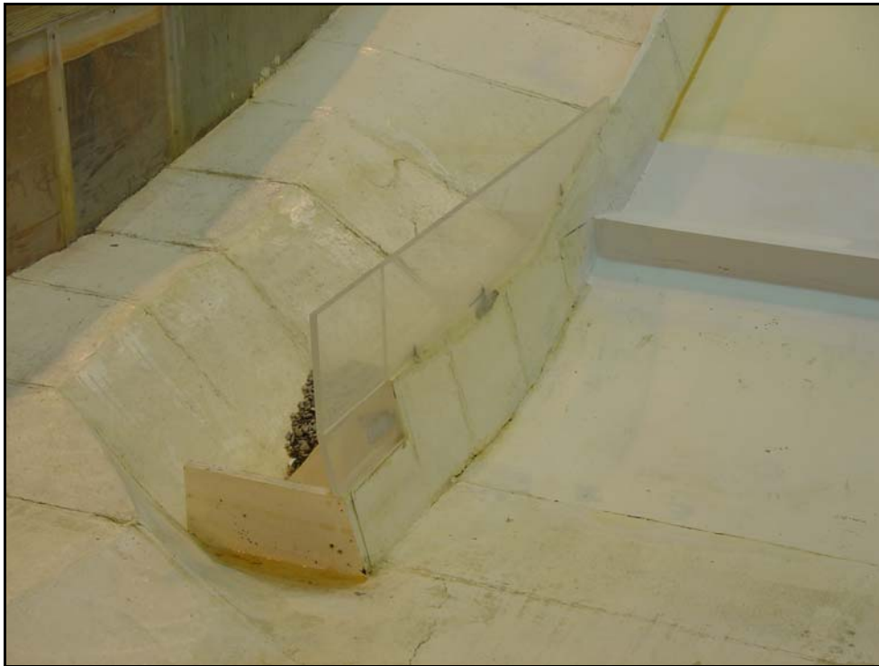
Figure 3-12. Photograph of the right bank training wall extension
