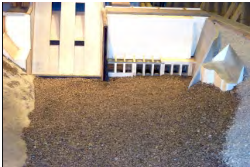
Figure 4.21. Looking upstream after 13.3 kcfs per crest gate
