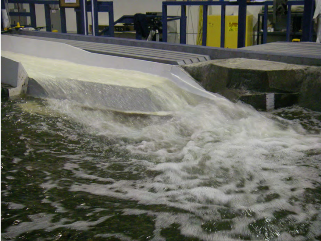
Photo 6.2.12 Deflector 14, 40,000 cfs, Low Tailwater, 3-Bay Operation
