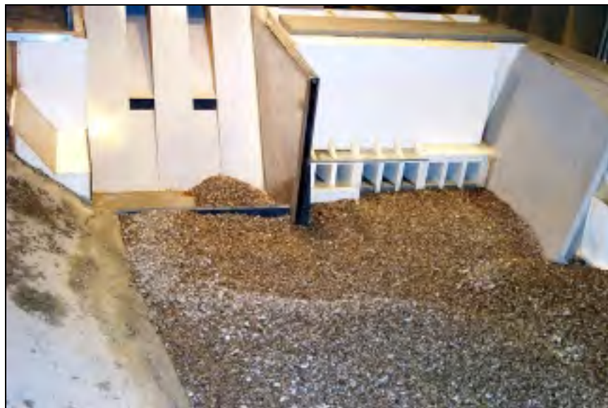
Figure 4.9. Looking upstream after 15 kcfs per sluiceway bay
