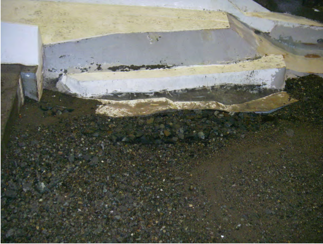
Photo 6.2.21 Rip rap test, Deflector 21, 70,000 cfs, 4'-6' rip rap.
