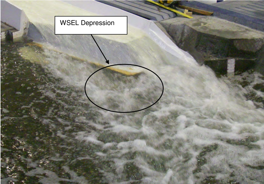
Photo 6.2.11 Localized water surface elevation depression located off northeast corner of the deflector.
