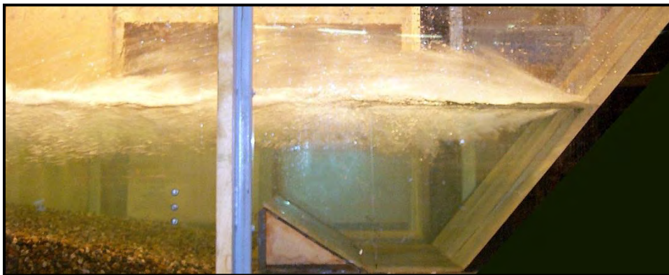
Figure G-5 Q=7.5 kcfs Per Sluiceway Bay with Tailwater Elevation of 1473.1 Feet
