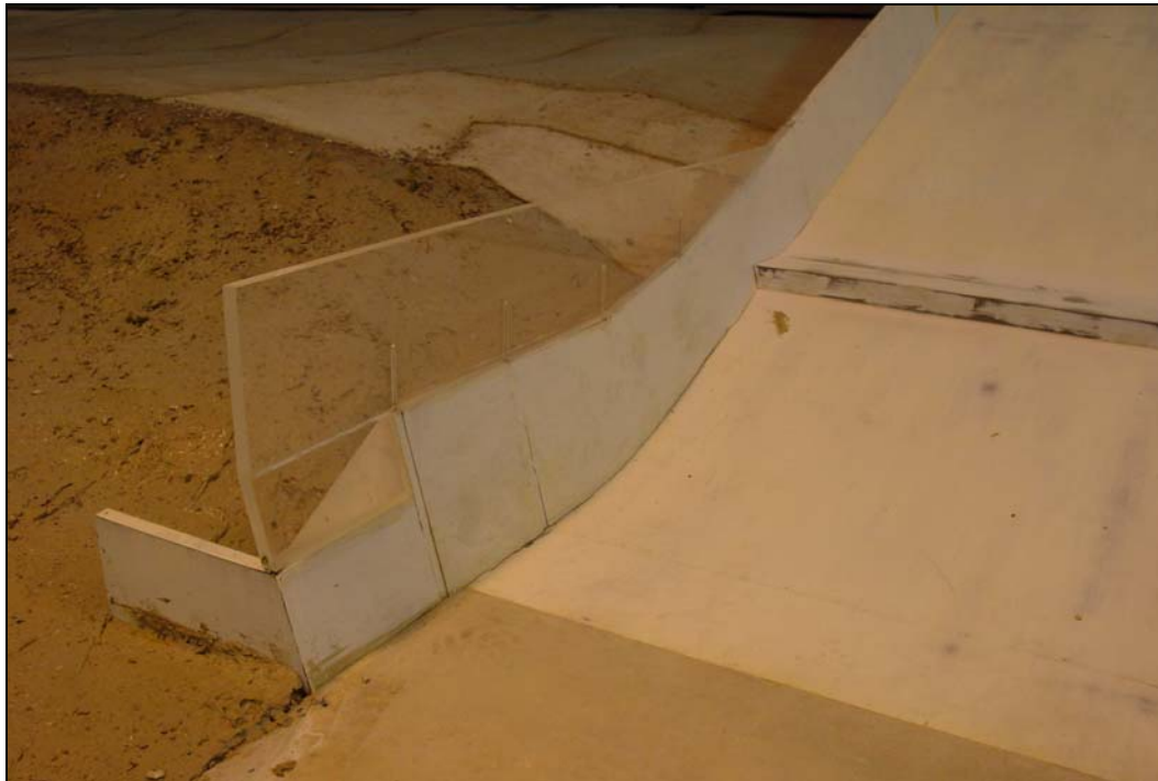
Figure 5-10. Photograph of the training wall extension as tested in phase two
