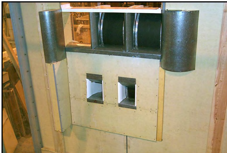
Figure 2.5 Upstream Face of 1:48 Model Headwall
