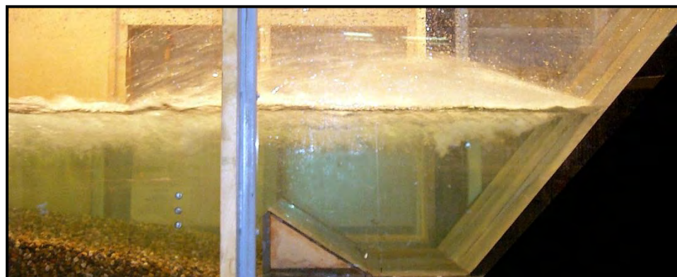
Figure G-3 Q=5.0 kcfs Per Sluiceway Bay with Tailwater Elevation of 1470.9 Feet
