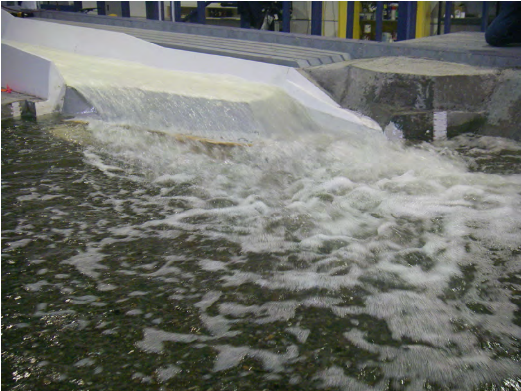
Photo 6.2.16 Deflector 19, 40,000 cfs, Low Tailwater, 3-Bay Operation
