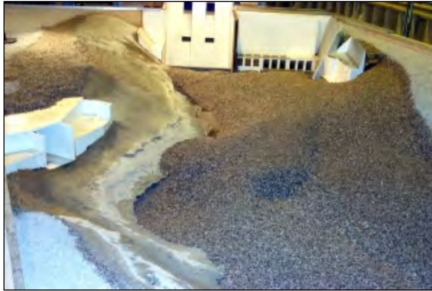
Figure 4.43. Looking upstream after 50 kcfs per crest gate
