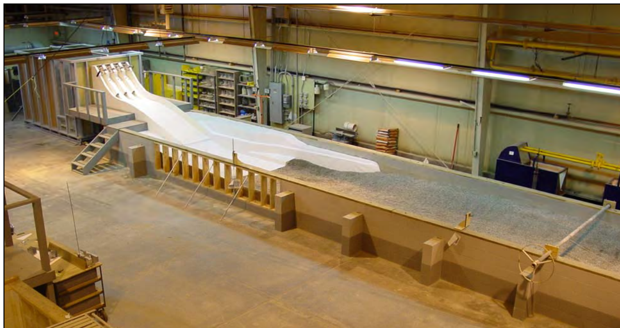
Figure 2-10. Photograph of the completed model basin
