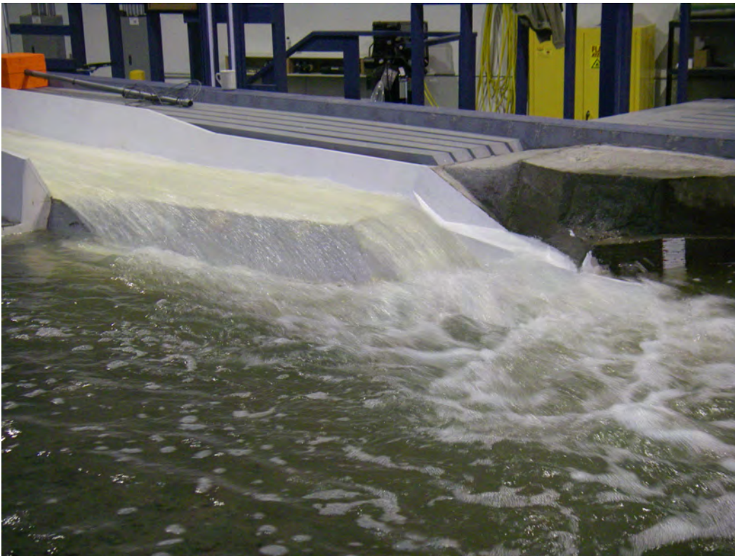
Photo 6.3.2 Final Documentation, Deflector 20, 40,000 cfs, 1699.1' tailwater.
