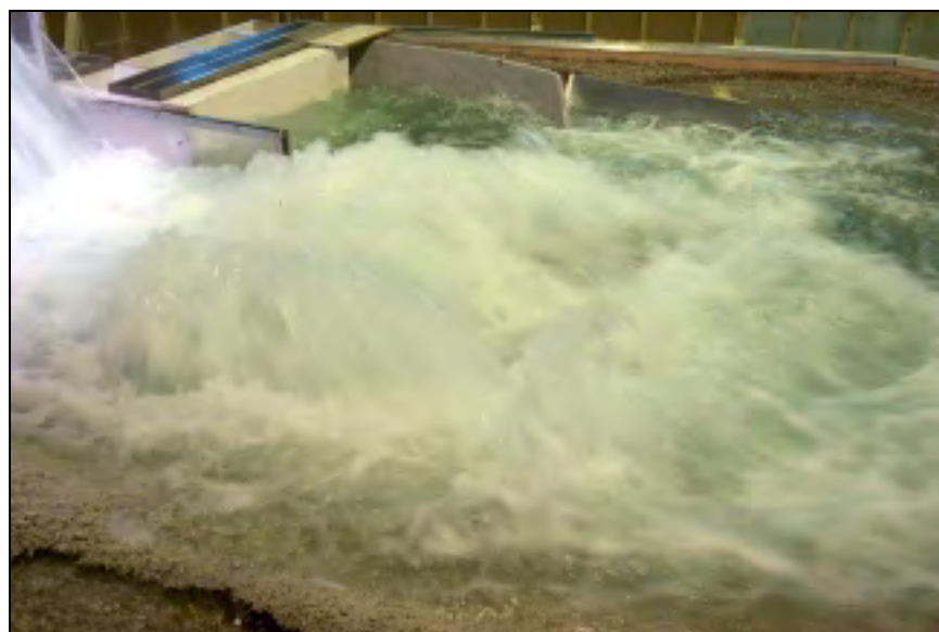
Figure 4.53. Boil created during design discharge
