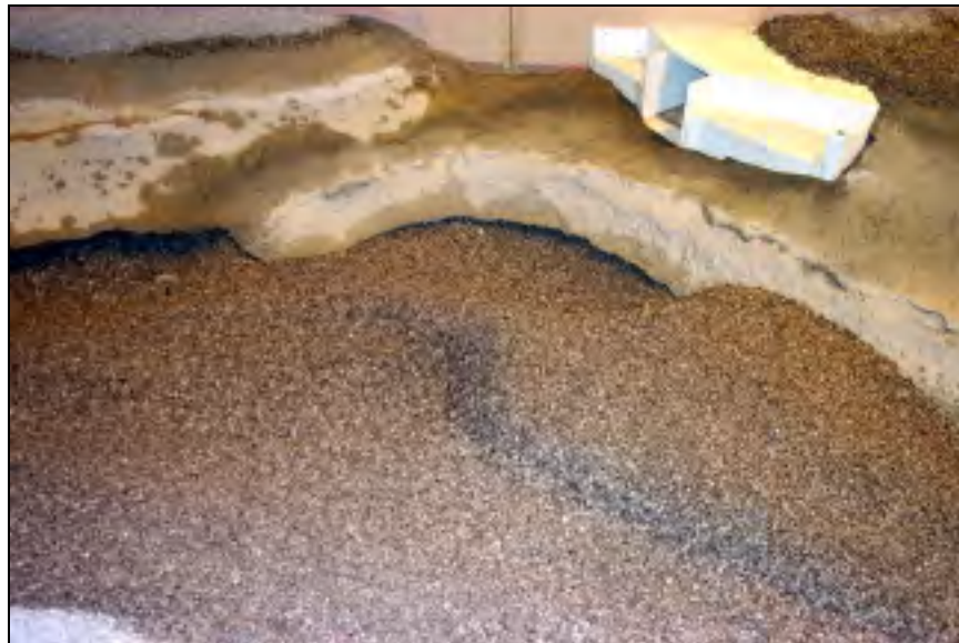
Figure 4.44. Diversion tunnel outlet scour patterns after 50 kcfs per crest gate
