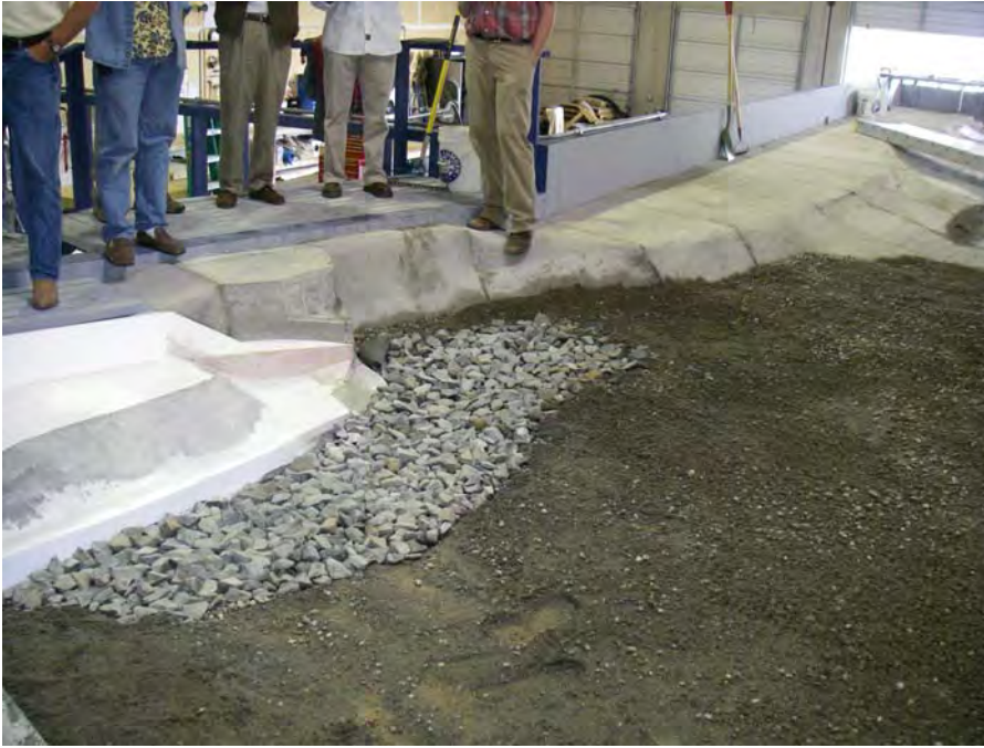
Photo 7 – Deflector with Riprap
