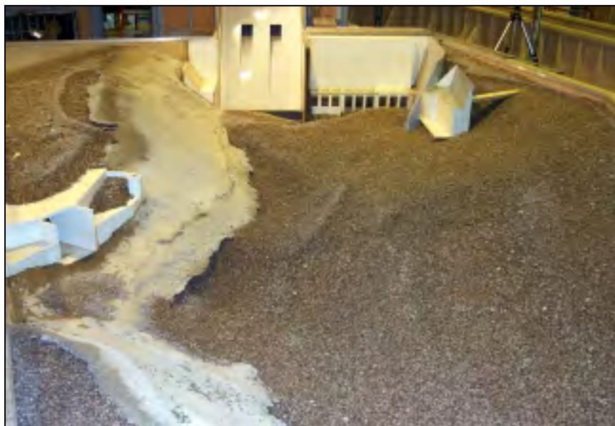
Figure 4.59. Looking upstream after design discharge event
