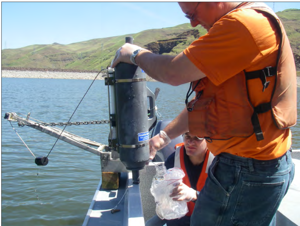
Figure 4. Niskin point-sampler used to collect water column samples in Brownlee Reservoir near Oxbow, Oregon, May 7–9, 2012.
