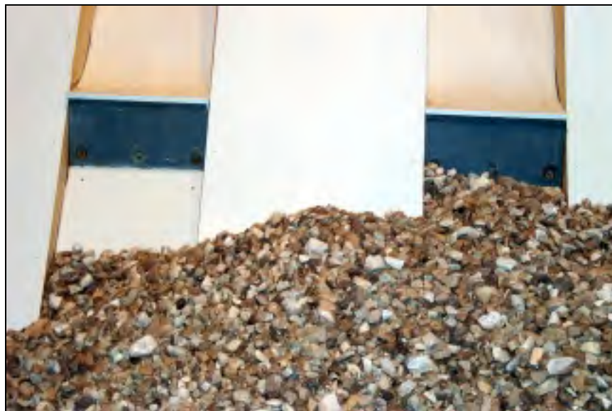
Figure 4.12. Rock pullback material touching vertical face of deflector
