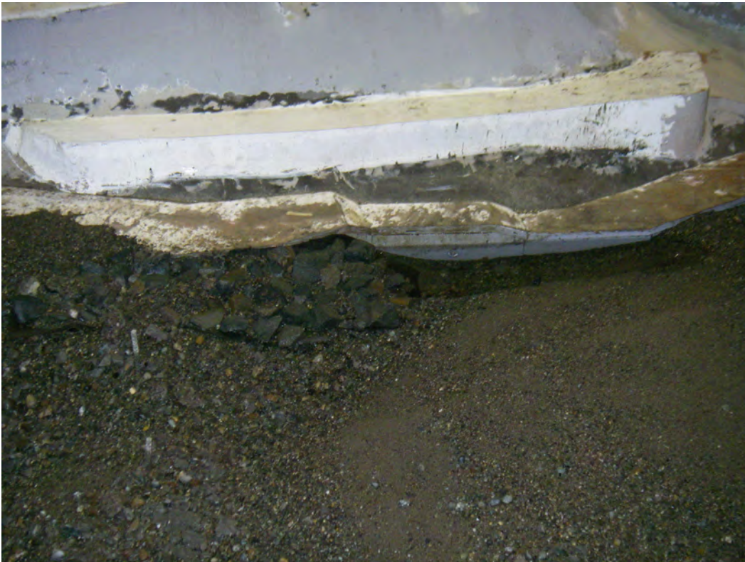
Photo 6.2.20 Rip rap test, Deflector 21, 70,000 cfs, 6'-10' rip rap.
