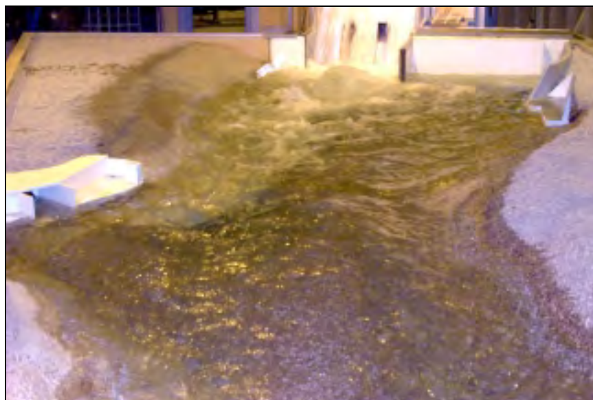
Figure 4.30. Looking upstream during 30 kcfs per crest gate
