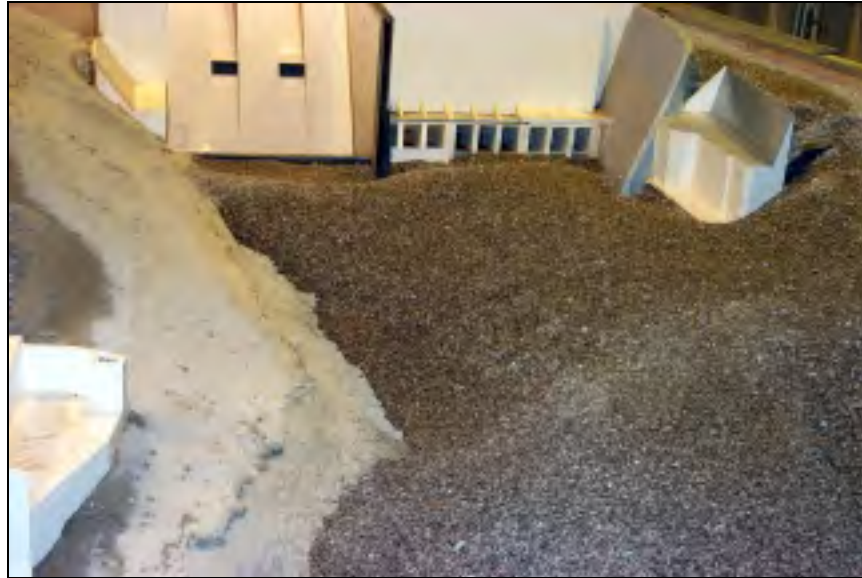
Figure 4.48. Looking upstream after 67 kcfs per crest gate
