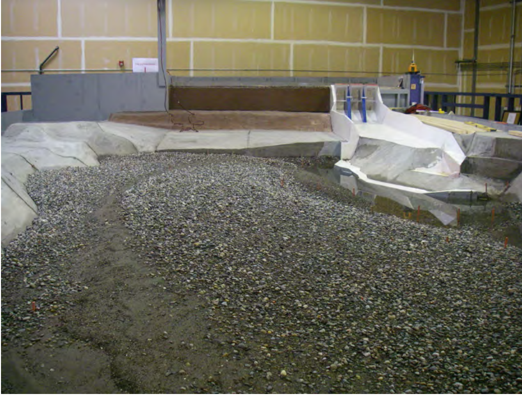
Photo 4.1 Oxbow physical model with dry mobile bed.
