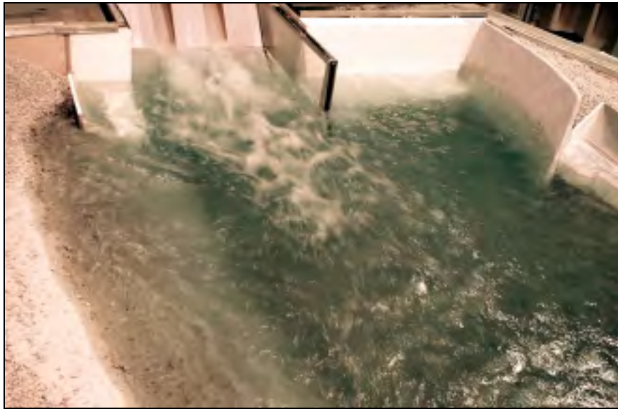
Figure 4.4. Sluiceway jets at 5 kcfs per bay
