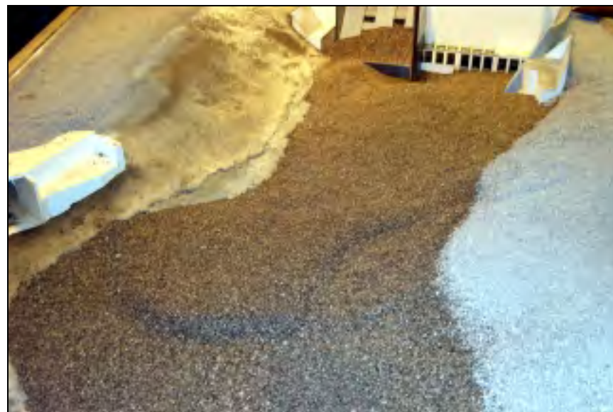
Figure 4.15. Erosion patterns after 20 kcfs per sluiceway bay
