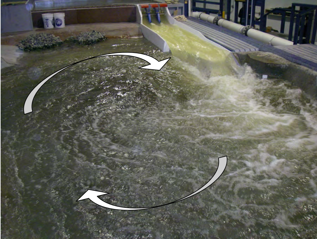
Photo 6.1.9 Baseline, 150,000 cfs, looking at left bank, circulation cell flow pattern shown.
