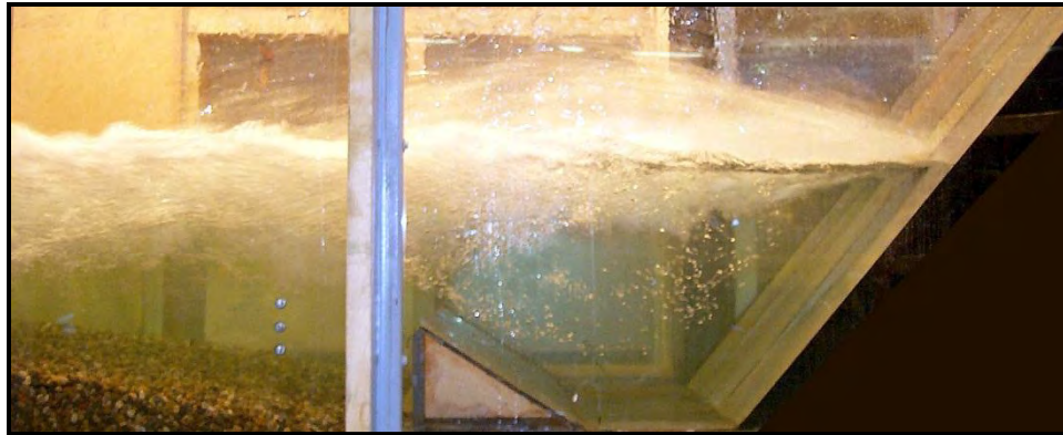
Figure G-7 Q=10.0 kcfs Per Sluiceway Bay with Tailwater Elevation of 1474.9 Feet
