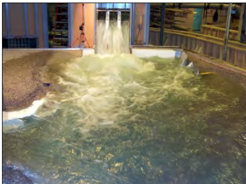
Figure 4.64. Looking upstream at design discharge with deflectors
