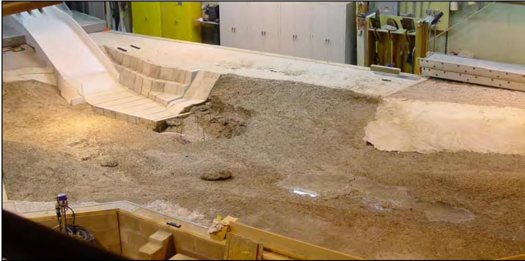
Figure 4-7. Photograph of the bed after the scour test with deflector (IP-3D-14)
