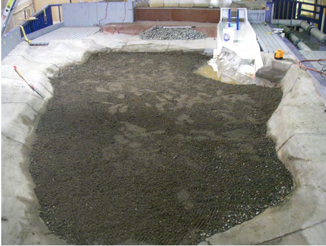
Photo 4.3 Oxbow physical model mobile bed, looking overhead..
