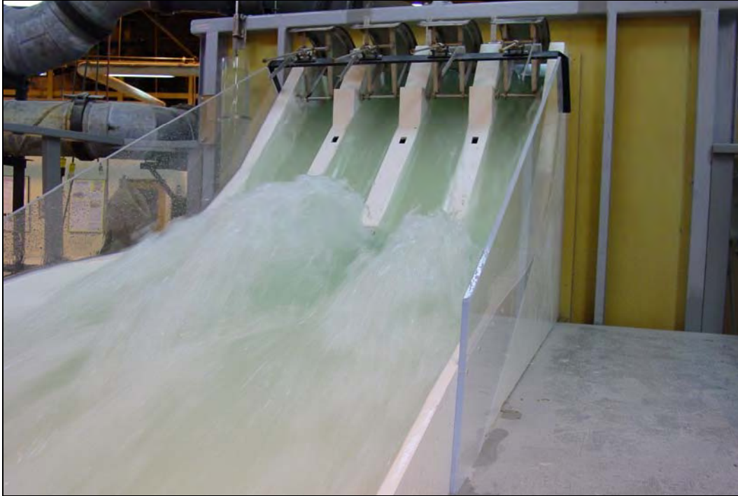
Figure 4-10. Photograph of the spillway chute during the PMF scour test
