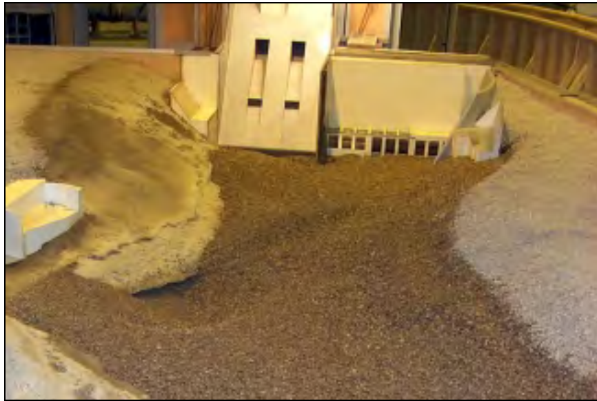
Figure 4.31. Looking upstream after 30 kcfs per crest gate
