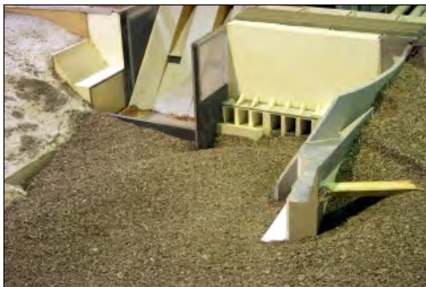
Figure 4.69. Scour and pullback near rightbank bedrock layer
