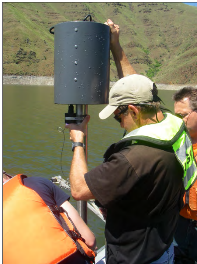
Figure 5. Ballchek™ bed-sediment core sampler used in Brownlee Reservoir near Oxbow, Oregon, May 7–9, 2012.
