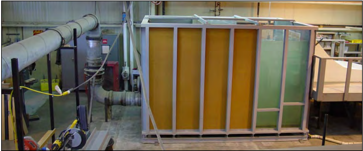
Figure 2-2. Photograph of the headbox and inflow pipe
