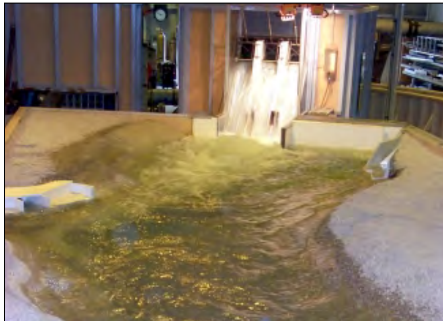
Figure 4.35. Looking upstream during 40 kcfs per crest gate
