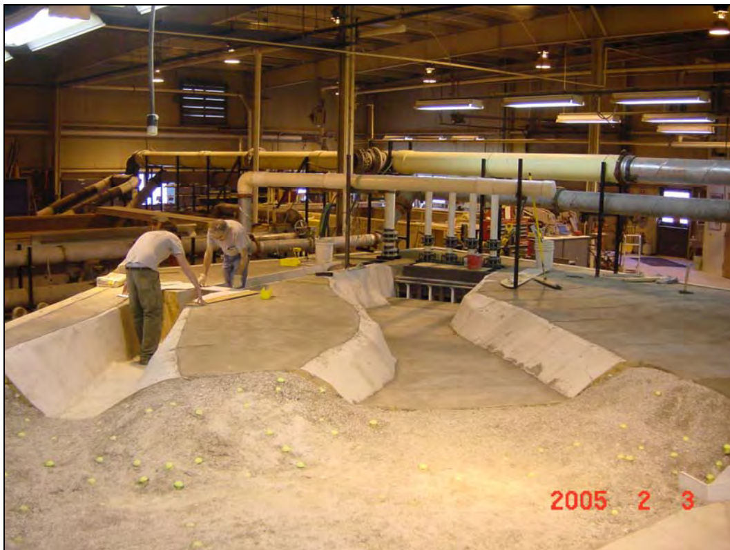
Figure 2-12. Photograph of completed bathymetry near the powerhouse
