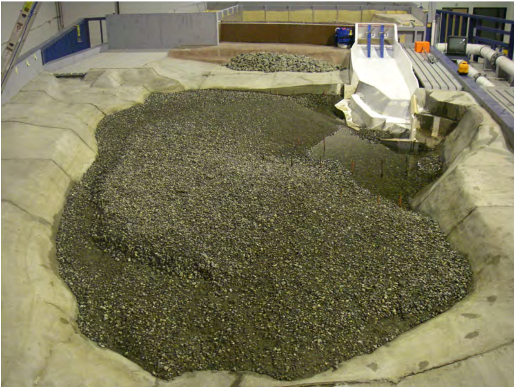
Photo 6.3.6 Final Documentation, Deflector 20, Mobile bed after 70,000 cfs erosion test.
