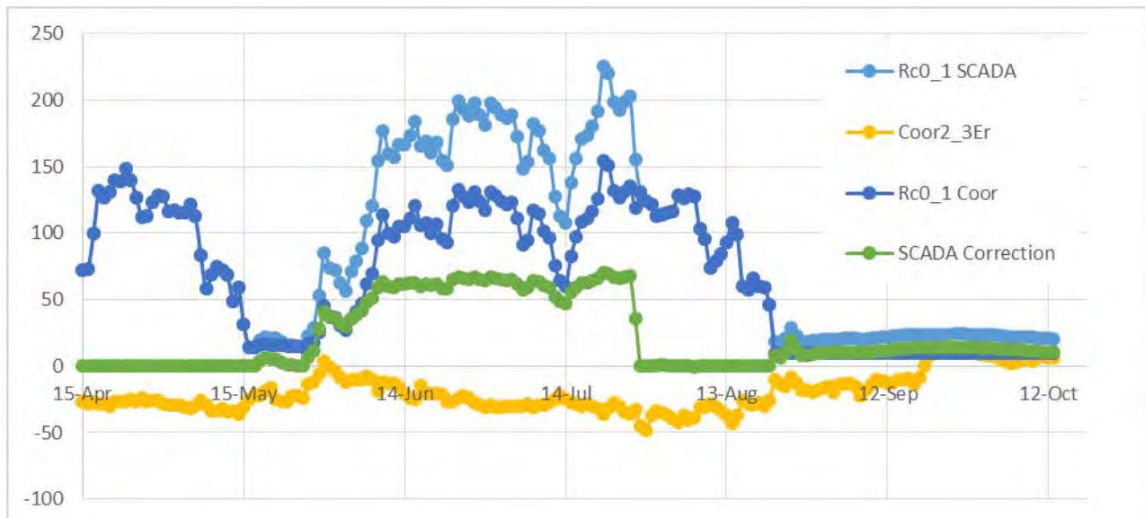
Figure A-1. Raw SCADA data (Rc0_1 SCADA), “corrected” SCADA including manual changes, calculated error at Rc3_3 (Coor2_3Er), and SCADA correction.
