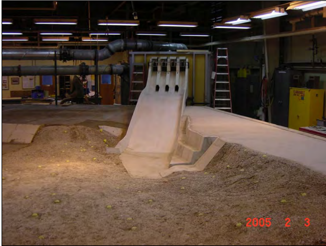
Figure 2-13. Photograph of completed bathymetry near the spillway
