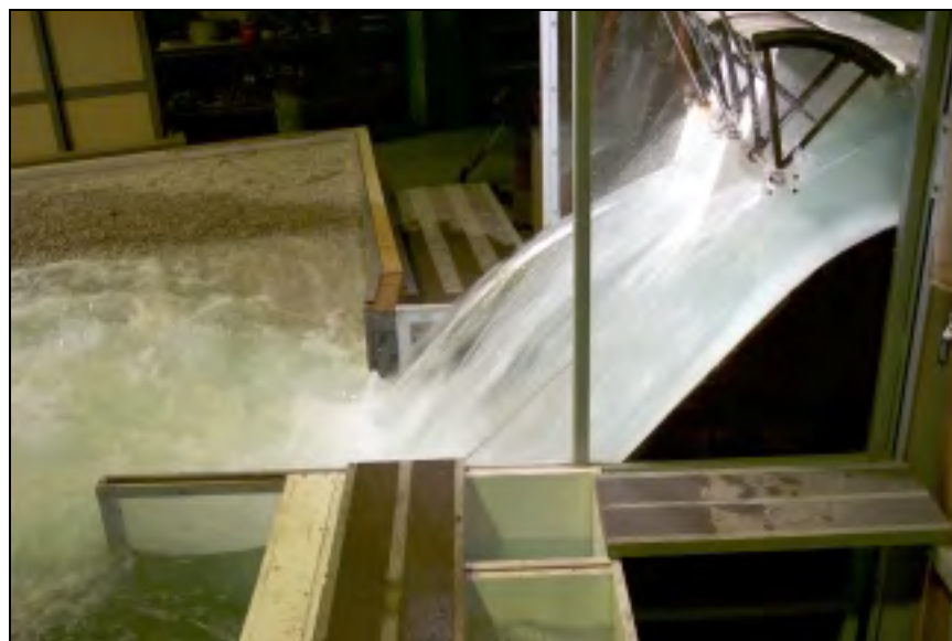
Figure 4.63. Spillway jets during design discharge
