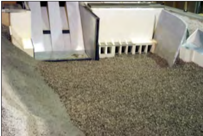
Figure 4.18. Looking upstream after 5 kcfs per crest gate
