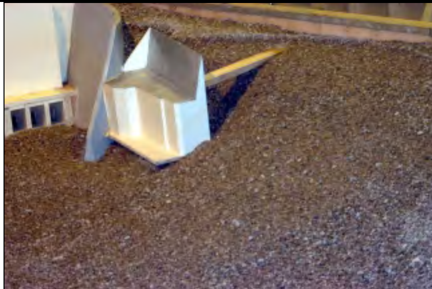
Figure 4.58. Wave erosion and undermining around fish ladder entrance
