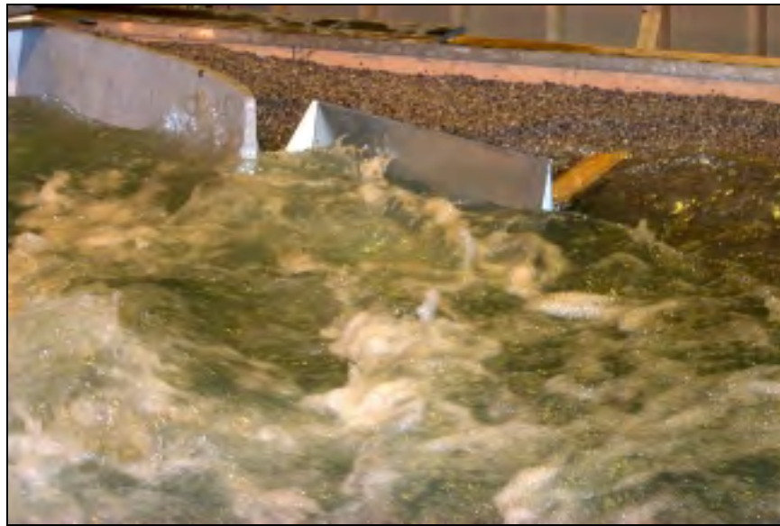
Figure 4.65. Waves breaking over fish ladder entrance
