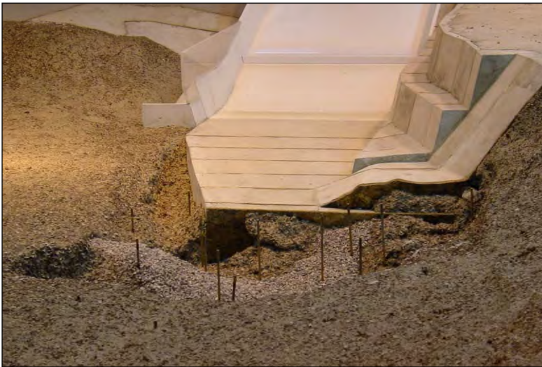
Figure 4-8. Primary scour hole looking upstream to apron after the scour test with deflector (IP-3D-14)
