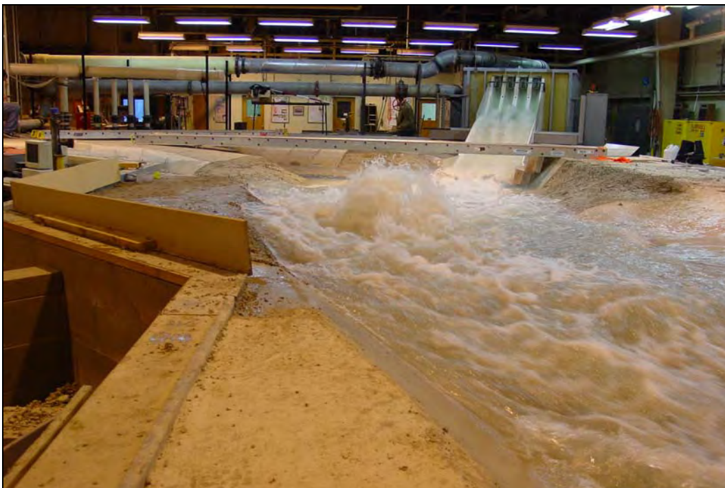
Figure 4-11. Photograph of the downstream reach during the PMF scour test
