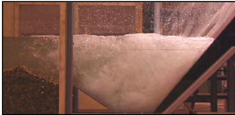
Figure 4.3 Baseline Condition with No Deflectors
