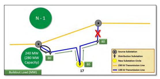
While 138 kV transmission lines typically have a capacity 200 MW, the sections of transmission lines that connect to the source substations can be rebuilt with larger conductor so that they have a capacity of 280 MW.
