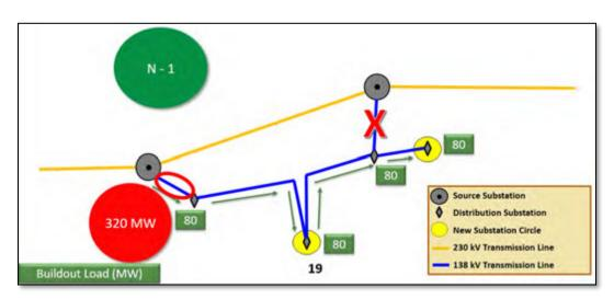
In this scenario, the section of transmission line circled in red would exceed the capacity of the larger conductor which has a rating of 280 MW.
