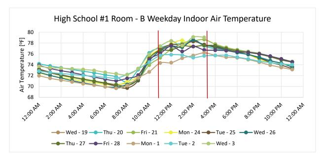
Figure 4: The indoor temperatures measured at the one classroom that showed thermal comfort
