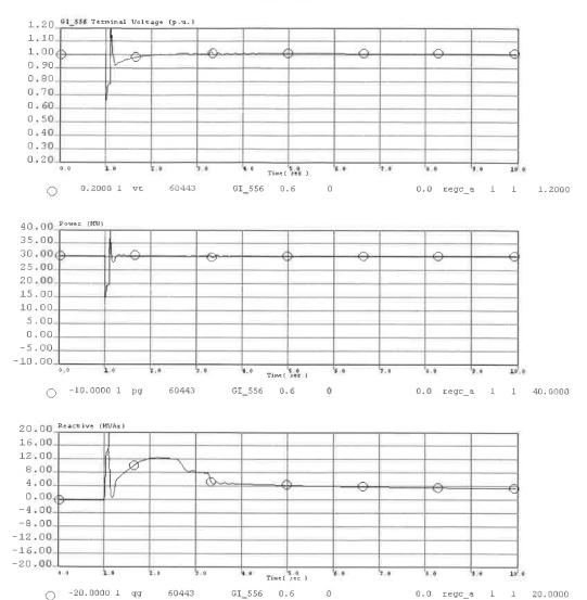
Loss of Brasada-HEPASOL2 115kV Line 3ph fault at HBASOL2 115kV clear in 6.0 cycles 3witched Quartz 138kV Shunt Reactor at 2.25 seconds
