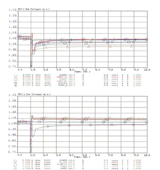
Hines 138kV Bus Differential - Clears Station 3LG fault at Hines 138kV clear in 6.0 cycles COMMENTS DUE TO DATA SUBMITTER BY July 13, 2018
