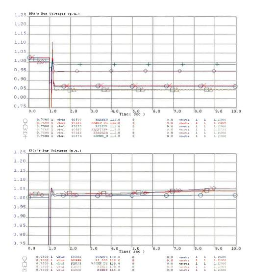
Loss of Mines-Marney 115kV Line 3pk fault at Mines 115kV clear in 6.0 cycles COMMENTS DUE TO DATA SUBMITTER BY July 13, 2018
