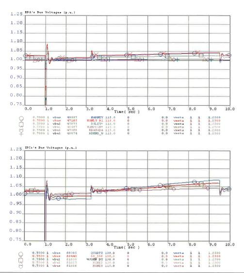
Loss of Quarts-N Powder-Brownlee 230kV Line and Quarts T231 230/129kV Transformer 3ph fault at Quarts 230kV Clear in 4.0 cycles 3witched Quarts 138kV 3kunt Capacitor at 2.25/8.50 seconds Trip LaGrande 230kV 3kunt Capacitor at 5.0 seconds COMMENTS DUE TO DATA SUBMITTER BY July 13, 2018 COMMENTS FROM DATA SUBMITTER BY July 13, 2018
