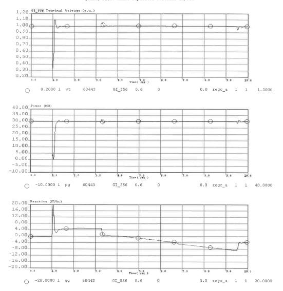
Loss of Quarts-N Powder-Brownice 230kV Line and Quarts T221 230/138kV Transformer
