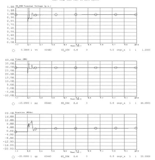
Loss of Brasada-Yew Ave-Redmond 115kV Line 3ph fault at Yew Av T 115kV clear in 6.0 cycles RAS: Trip 40 MW Harney Area Solar as 21.0 cycles
